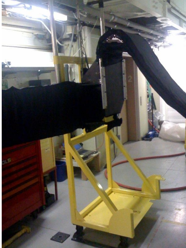
A new fiber transition mount will minimize risk to the fibers and improve safety and operations for the Hectospec and Hectochelle instruments.
