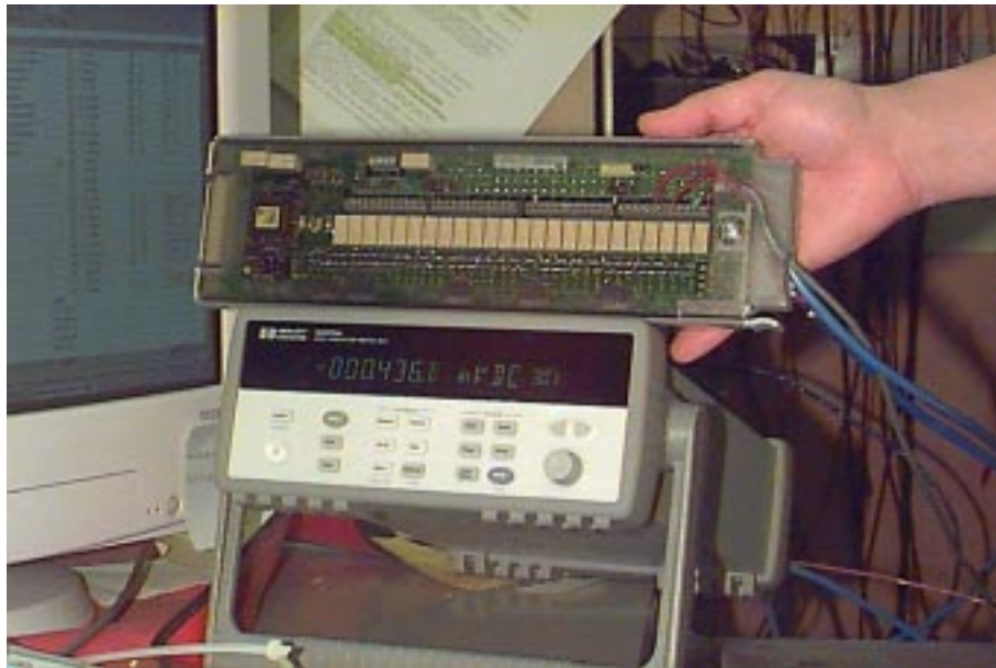
FIGURE 7. Thermocouple measurement electronics consisting of an HP 34970A data acquisition unit (lower) and HP 34901A armature MUX.
