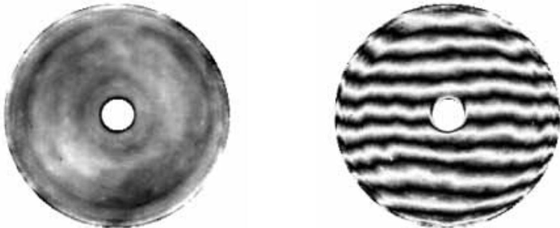
Figure 4. Gray-scale map of the mirror surface and synthetic interferogram for the MMT mirror with astigmatism and spherical aberration subtracted. The gray scale covers  $\pm 100$  nm of surface and the rms surface error is 35 nm. The interferogram is calculated for a wavelength of 531 nm.
