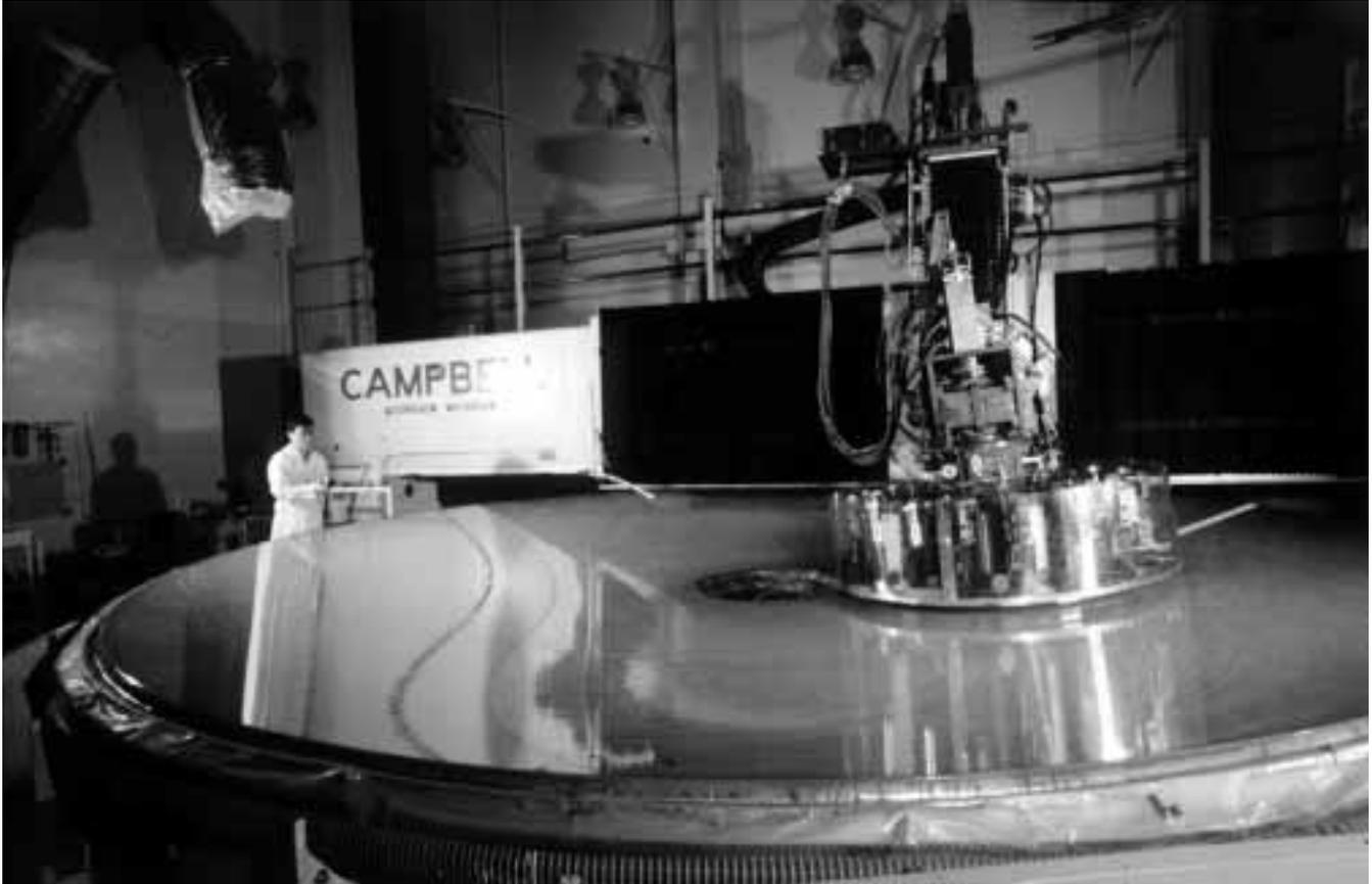
Figure 3. MMT primary mirror being polished.
