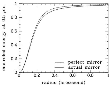
Figure 8. Encircled energy as a function of radius for the Magellan mirror and for a perfect mirror. Top: in perfect seeing. Bottom: in seeing of  $0.25''$  FWHM.
