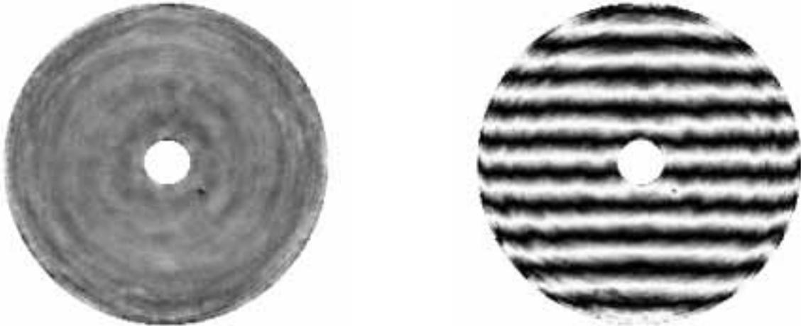
Figure 6. Gray-scale map of the mirror surface and synthetic interferogram for the Magellan mirror with astigmatism and spherical aberration subtracted. The gray scale covers  $\pm 100$  nm of surface and the rms surface error is 14 nm. The interferogram is calculated for a wavelength of 531 nm.
