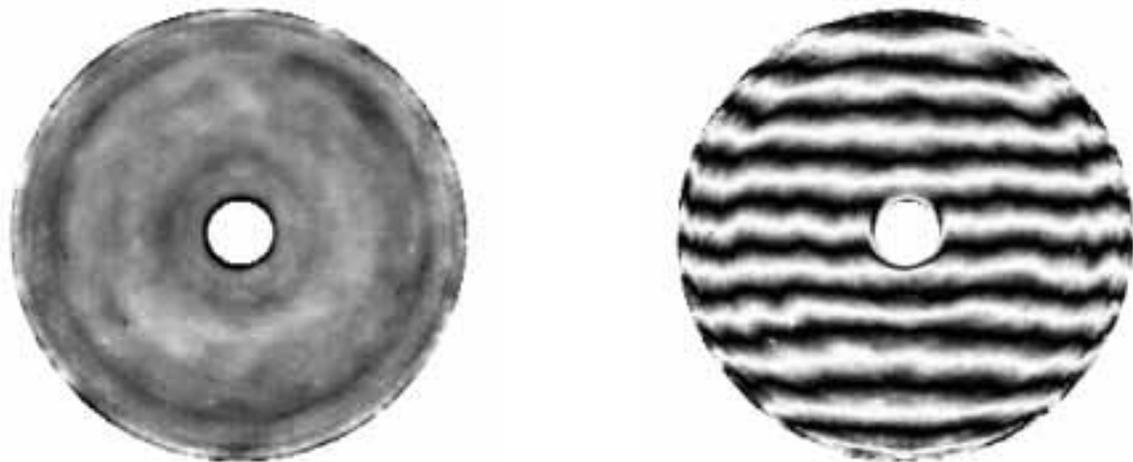
Figure 5. Same as Figure 4 except that two additional flexible bending modes have been subtracted. The rms surface error is 26 nm.
