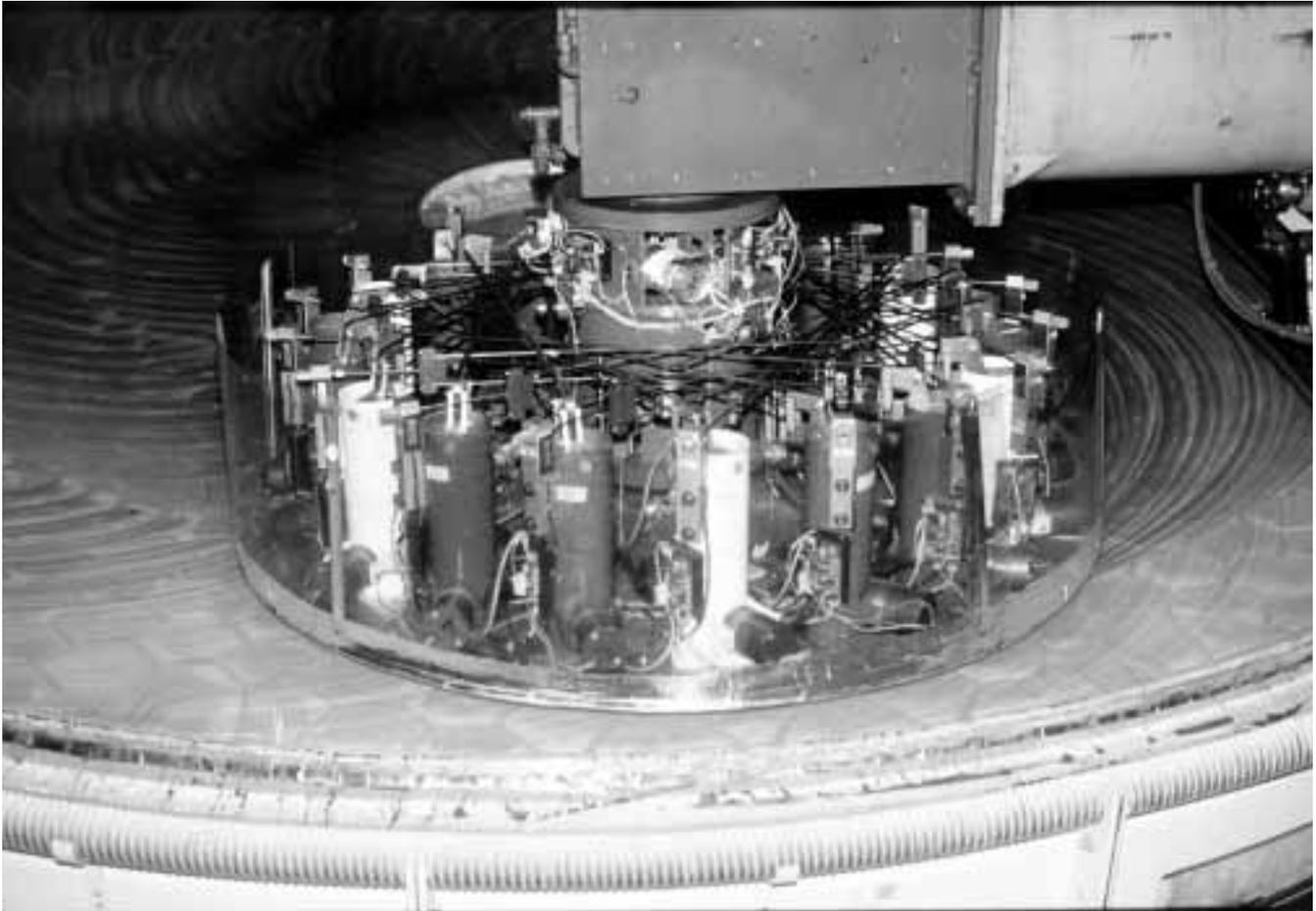
Figure 2. Stressed lap in use on the MMT mirror.
