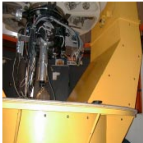
Figure 2: The interferometric Hartmann wavefront sensor attached to the VATT.
