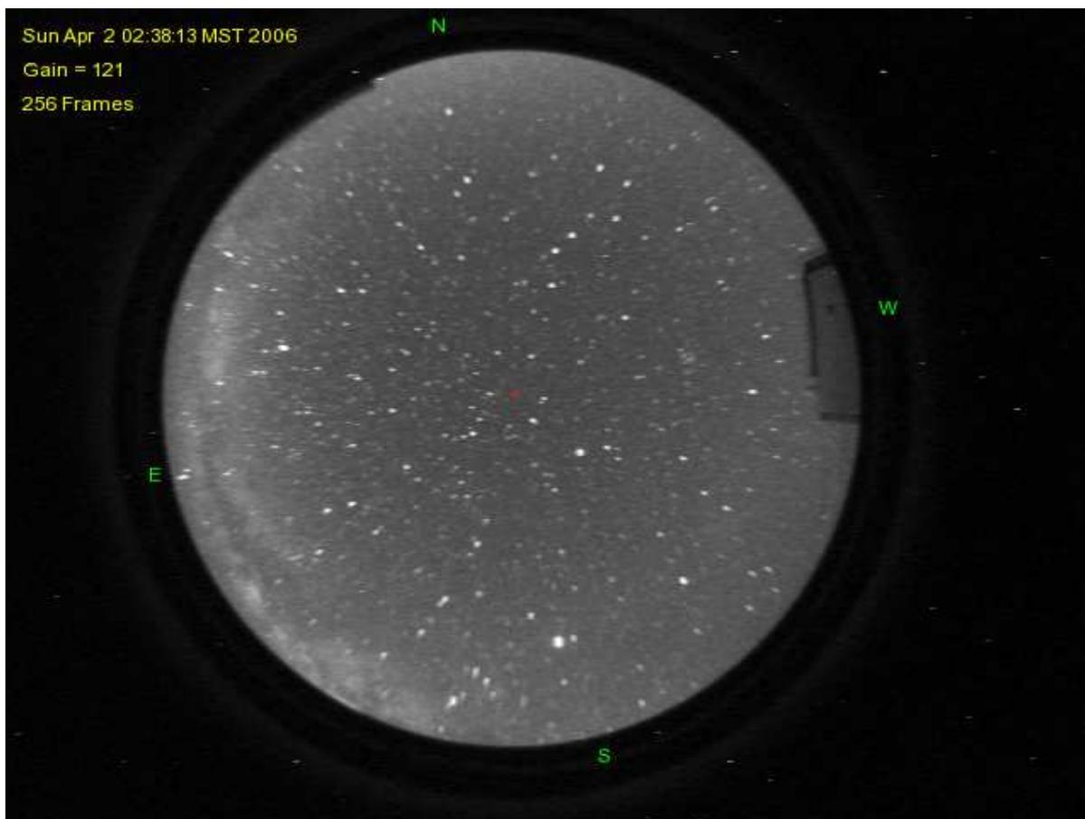
**Figure 3.** Representative image taken by the MMT All-Sky Camera on a clear, moonless night. The timestamp of the image and the camera configuration information are shown in the upper left corner of the image. The cardinal directions are plotted on the image for reference along with a red cross at the position that corresponds to where the MMT is pointing.
