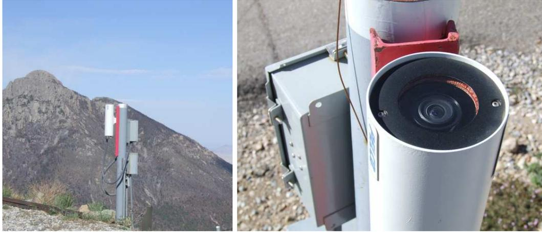
**Figure 1.** Pictures of the installed sky camera system. The image on the left shows the enclosure and junction box mounted on a pole at the east end of the summit parking lot. The image on the right shows the entrance window of the enclosure.
