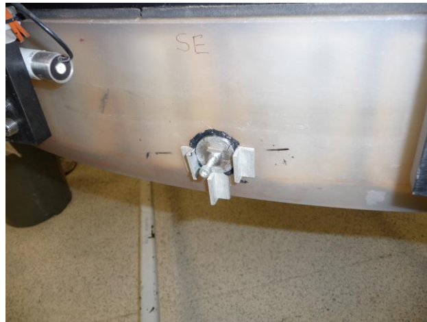
Figure 1. Tangent rod puck installation brackets
