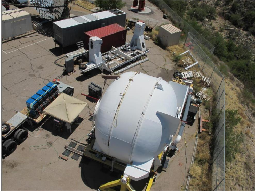
Figure 2. The bell jar assembly (front, extension, and rear) used to conduct coating tests at the base camp. The pumping trailer is shown in the top portion of the photo, and the welders (blue) are on the left.
