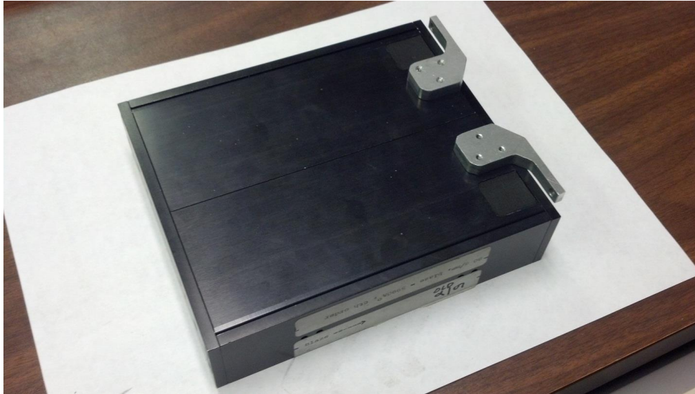
Figure 4. Old grating cell with new door blocks installed.
