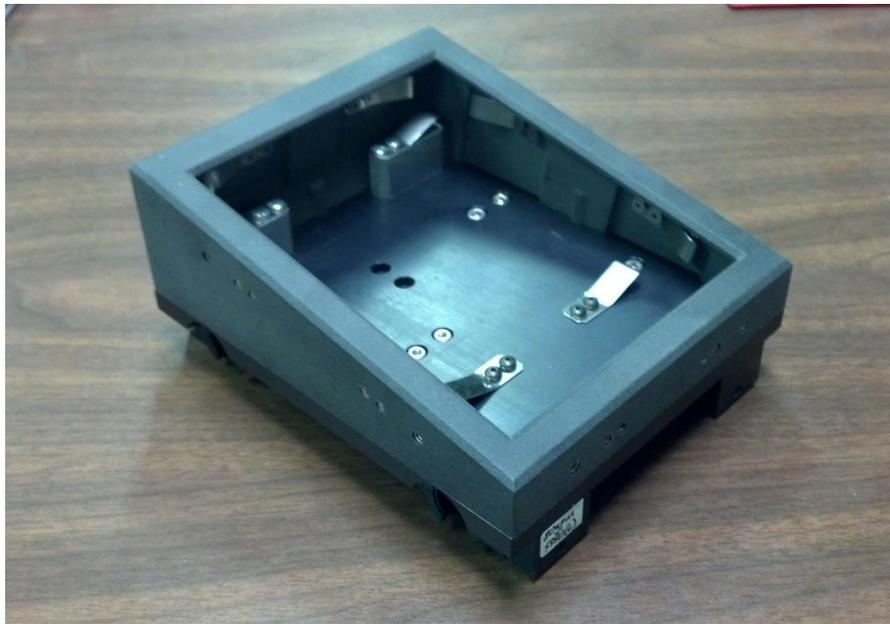
Figure 3. New grating cell with backplate and positioning springs attached.
