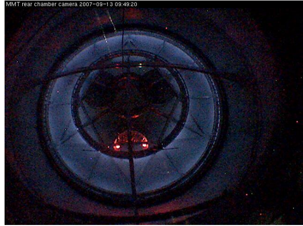
Figure 2: Oxygen rich (left) then Argon rich (right) gas glows in the 6.5-m coating chamber during the glow discharge (ion bombardment) cleaning phase, immediately before aluminum deposition.
