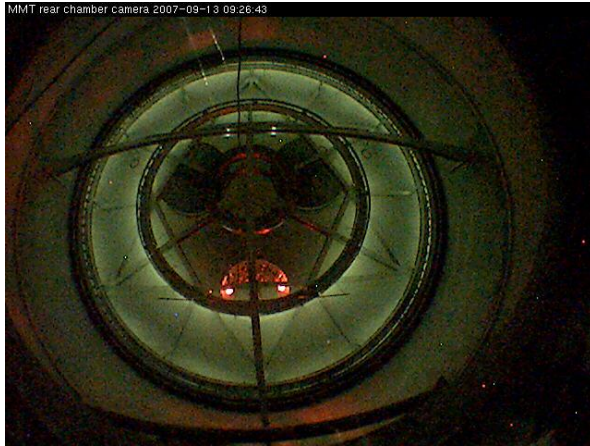
Figure 2: Oxygen rich (left) then Argon rich (right) gas glows in the 6.5-m coating chamber during the glow discharge (ion bombardment) cleaning phase, immediately before aluminum deposition.
