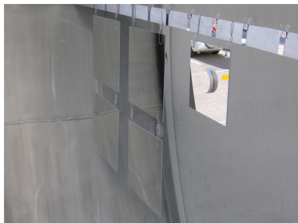
Figure 3: Forty-five microscope slides mounted on radial arms for measurement of aluminum thickness distribution (left). A Borofloat glass plate with 4" diameter dummy Hartman mirror (right).
