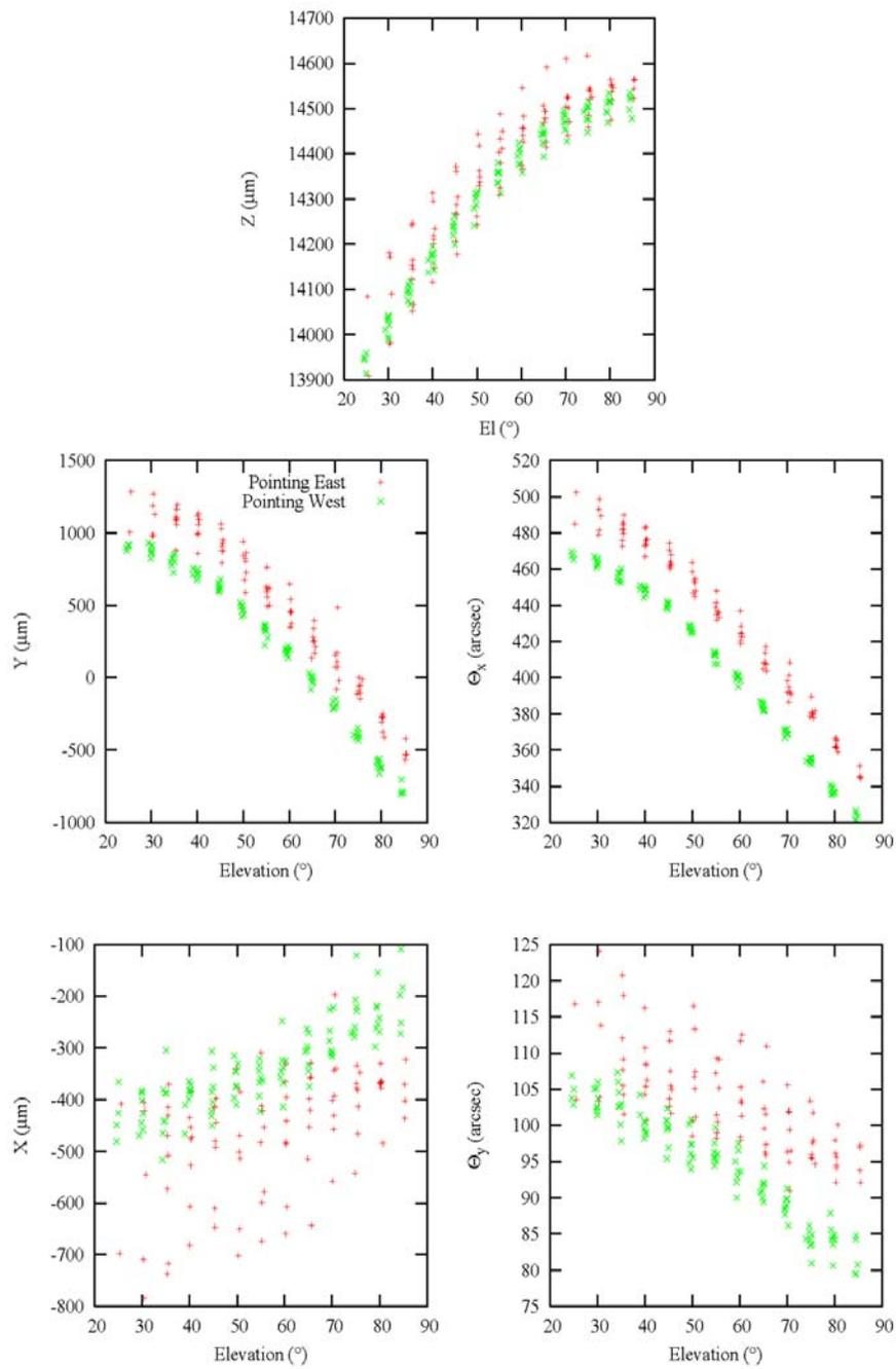
Figure 2: Engineering data from the night of April 25-26, 2006, taken while pointing west (green points) and then pointing east (red points).
