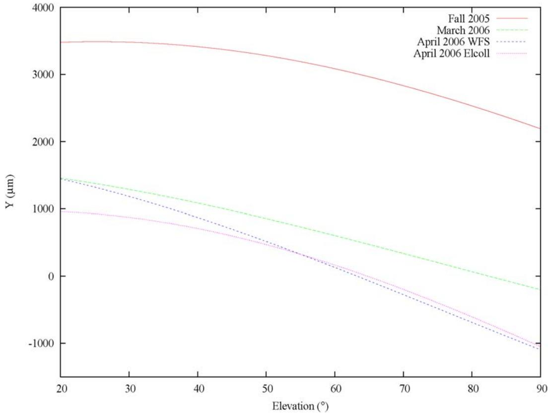
Figure 3: *Y vs. Elevation relations determined at different times between November 2005 and late April 2006. Note the very large offset of about 2.5 mm between November 2005 and all of the results from 2006.*
