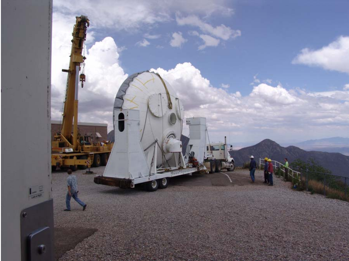
MMTO's 7-m diameter aluminumizing belljar leaves the Mt. Hopkins summit for the FLWO basecamp, then to the Steward Mirror Lab where it will be mated to a new "back" belljar of the same design to form a "new" complete 7-m vacuum vessel.
