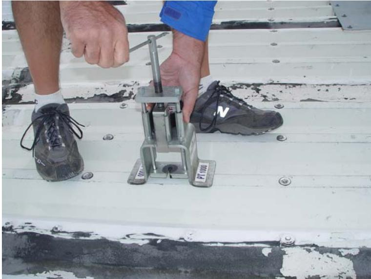
Figure 6: This picture shows Ron Olsen (Rain-Tite Roofing) measuring the pull-strength of typical fasteners used to attach the new roofing material. The pull strength of each fastener was typically 500 lbs. This is more than adequate to meet our extreme wind loads. Photo by Shawn Callahan (MMTO).
