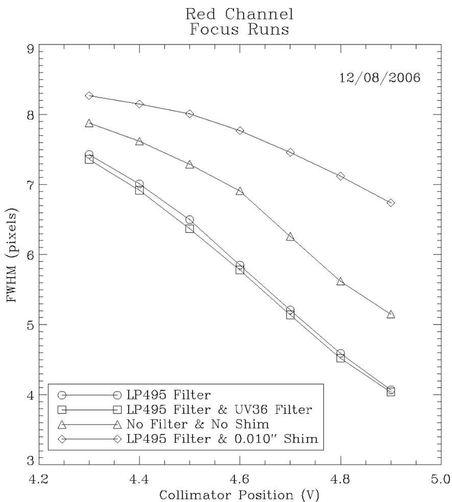
Figure 4: FWHM of comparison lamp lines
