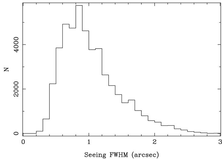
Figure 8: Histogram of 48,085 seeing measurements made by the f/9 and f/5 Shack-Hartmann wavefront sensors since March 2003.
