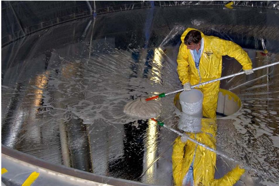
Soapsuds-dabbing (no-scratch) mirror wash technique is demonstrated by J. T. Williams on the 6.5-m (256 inch) diameter primary mirror.
