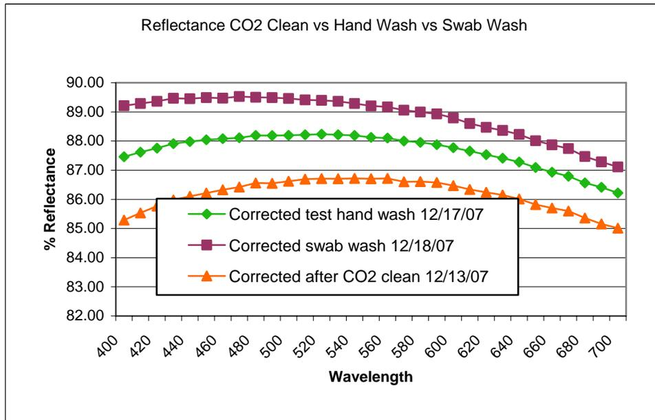
Figures 1 and 2: Optical scattering and reflectance results of final wet soap dabbing, washing, and drying are compared with hand cotton pads and routine CO<sub>2</sub> snow techniques. Measurements were made using a Minolta CM-2002 spectrophotometer.
