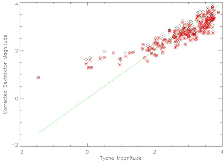
Figure 7: Plot of average measured versus catalog magnitudes for a set of stars from the Yale Bright Star Catalog observed over the course of a clear night with the all-sky camera. The red points are corrected for a zero-point offset only, while the white points also include a correction for a color term. The green lines show a 1:1 correspondence. The effects of saturation become significant for stars brighter than first magnitude.
