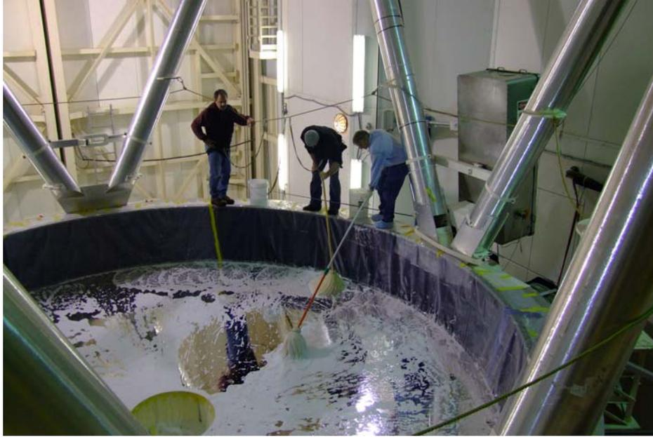
Figure 3: Brian Comisso and John Di Miceli join J. T. Williams in the first course dabbing and soaking of the 27-month old aluminum coating.
