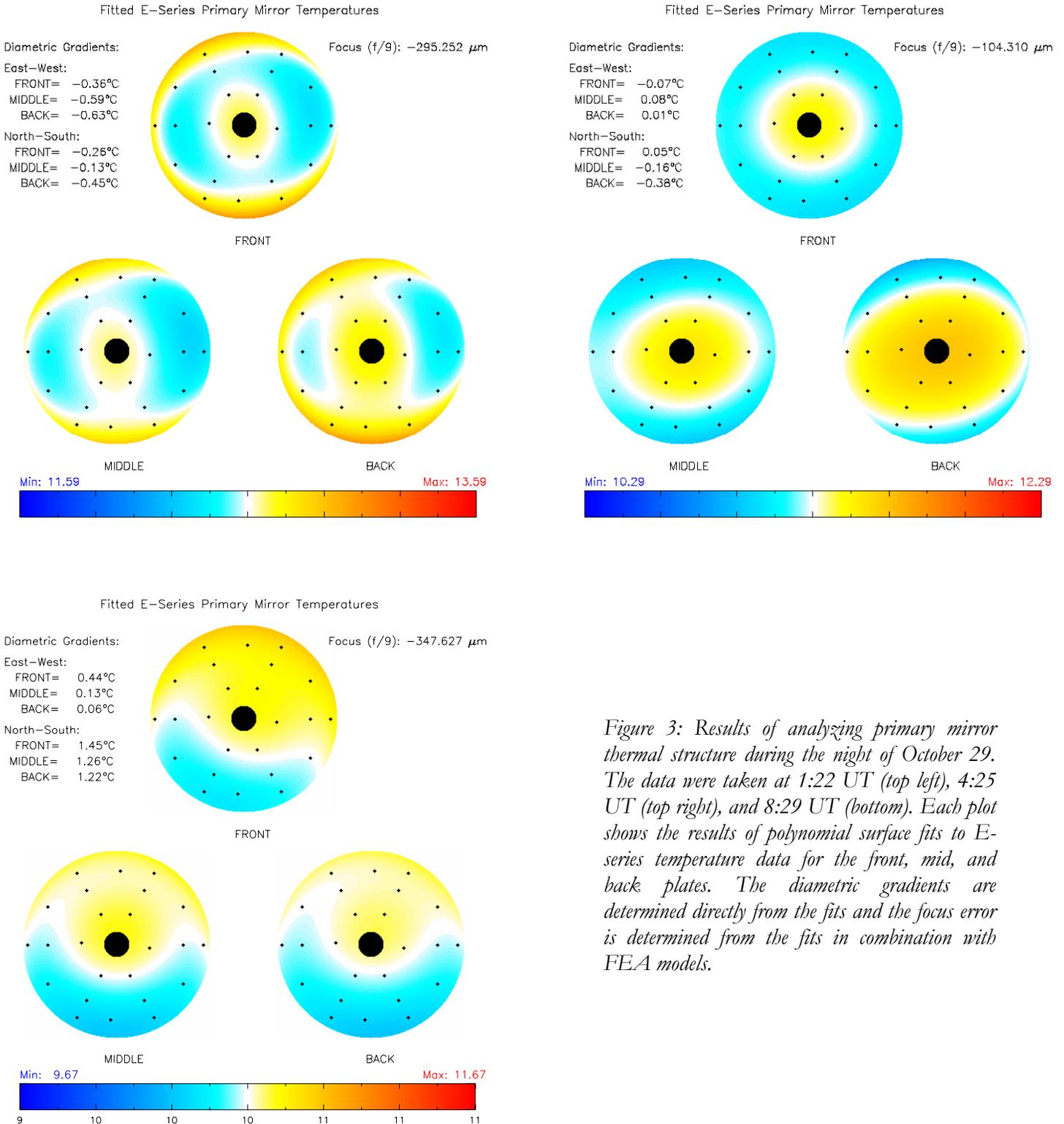
Figure 3: Results of analyzing primary mirror thermal structure during the night of October 29. The data were taken at 1:22 UT (top left), 4:25 UT (top right), and 8:29 UT (bottom). Each plot shows the results of polynomial surface fits to E-series temperature data for the front, mid, and back plates. The diametric gradients are determined directly from the fits and the focus error is determined from the fits in combination with FEA models.
