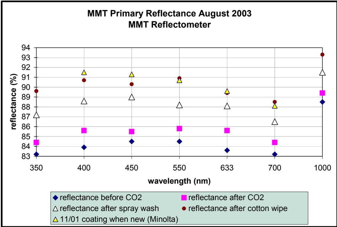
Figure 1. Reflectance at various stages of cleaning.
