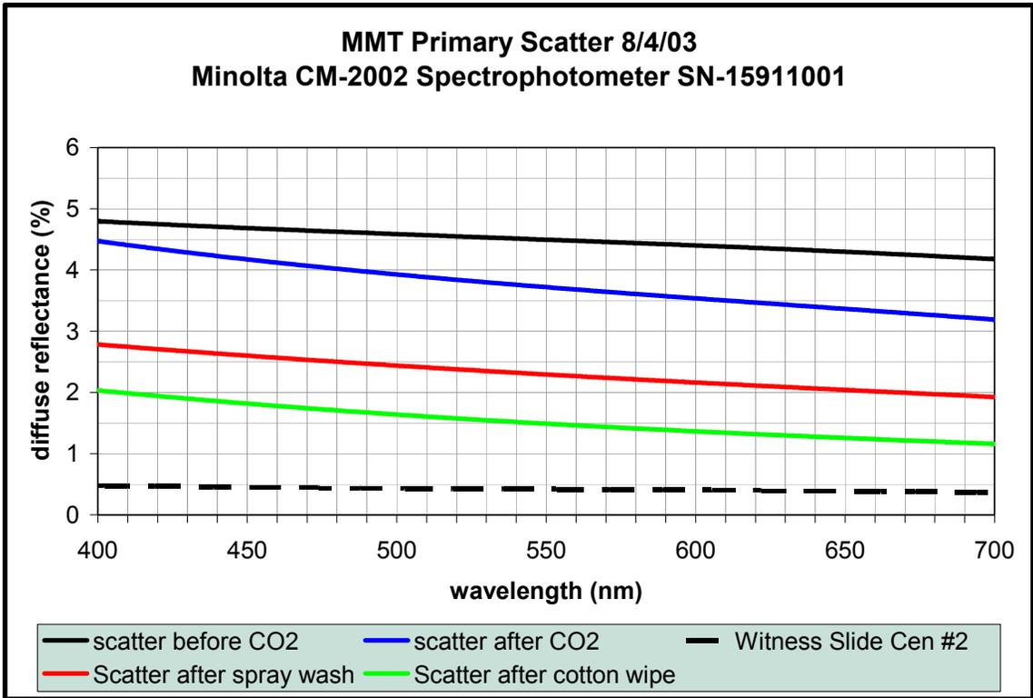
Figure 1. Scattering at various stages of cleaning.
