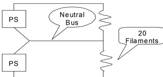
**Figure 1 Typical Filament Circuit (1 of 5)**
