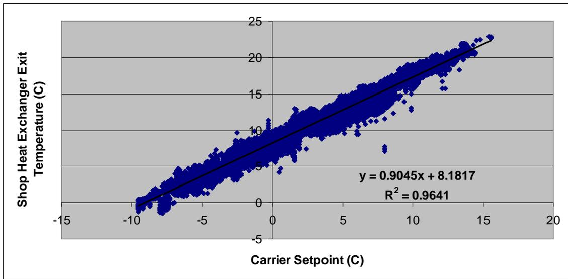
Figure 2. Linear regression at location “A,” using the “least squares” method, of the Carrier setpoint vs. shop heat exchanger exit temperature. See text for details.
