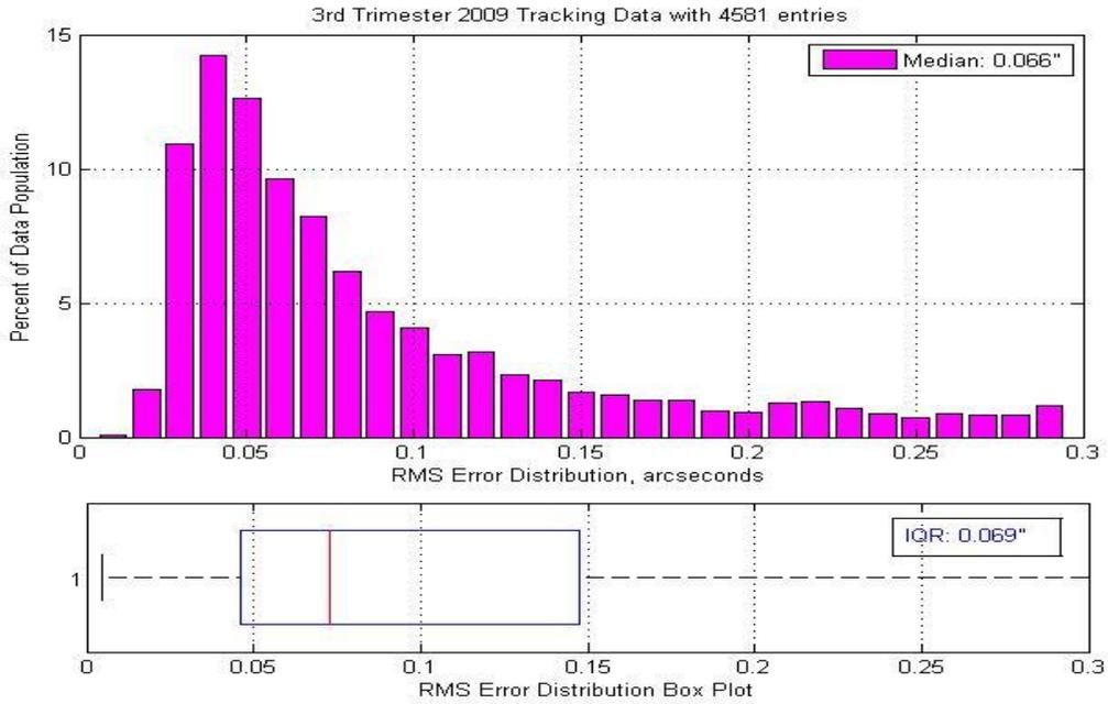
As earlier reported, there is also a lower limit to the tracking error that is related to velocity down to the absolute encoder quantization limit of 0.038\":
