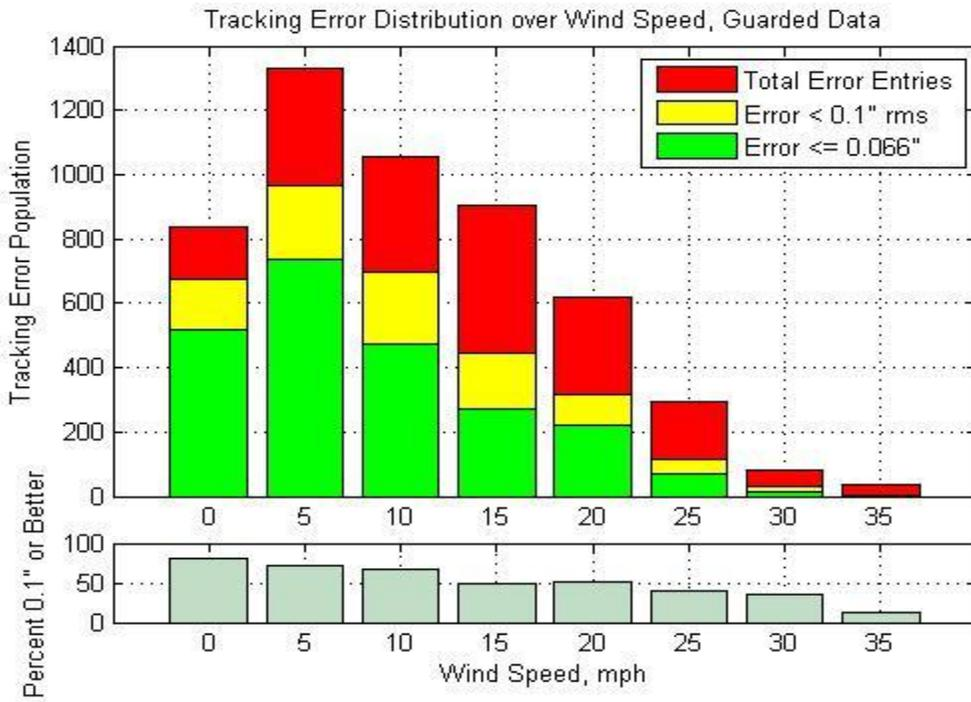
The error distribution can be combined, as shown below. In addition, we can see that low elevations away from the wind are also situations that produce better tracking:
