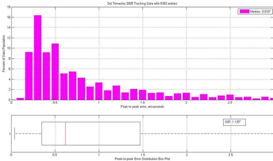
The `boxplot` routine records the outlier value for the RMS data as  $\sim 0.3''$ , so guarding the data by exclusion of those entries removes 582 members from the data set. We do this exclusion due to unwanted capturing of guider offsets and other step changes in the logged data that tend to contaminate the error statistics. This changes the RMS error distribution somewhat; the median RMS error then becomes  $0.066''$ , with an IQR of  $0.029''$ .
