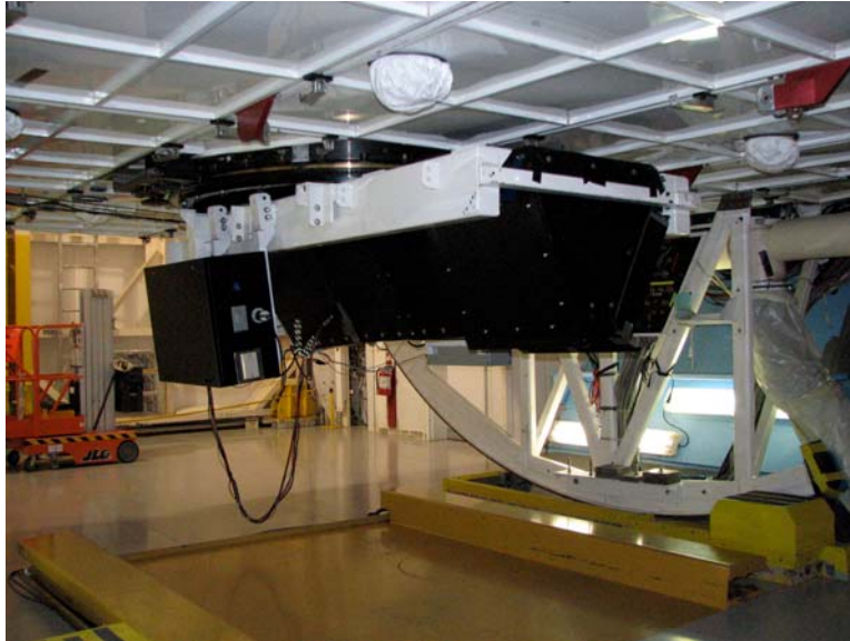
Figure 16: MAESTRO was mounted on the MMT for its first science run during April 2008. The end closest to the chamber shutters houses the injection optics, slit plate and dewar. At the opposite end is the prism and grating. MAESTRO can rotate to any given rotator angle as it utilizes the ADC and f/5 WFS.
