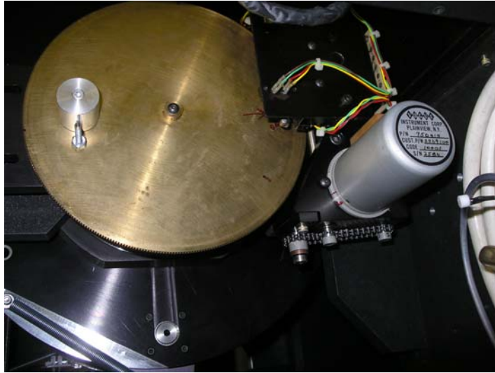
Figure 12: The brass worm wheel. The aluminum cylinder on the left triggers both the forward and reverse limit switches. The aluminum screw on the left triggers the optical indexer.
