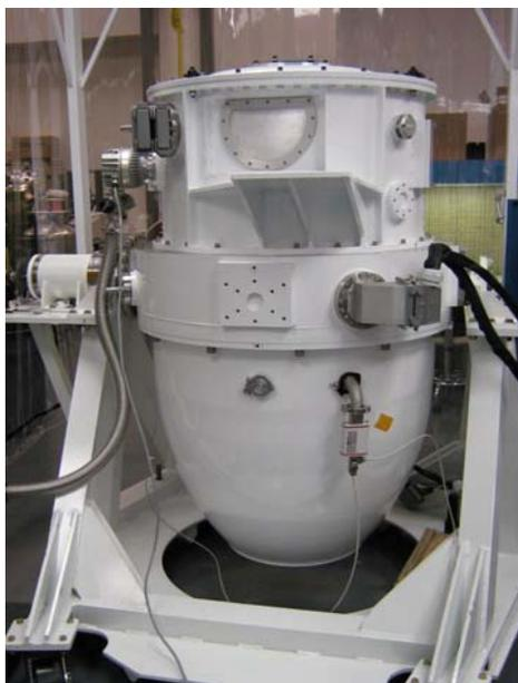
**Figure 15: MMIRS on its cart in the lab at the Cambridge Discovery Park. The lower half is the “camera dewar,” which houses the camera and collimator optics, grisms, filters, and detector. The top half is the “MOS dewar,” which contains the mask wheel and guide cameras. The two dewars are separated, but a gate valve allows the MOS dewar to be warmed up daily to interchange slit masks, while the camera dewar remains at operating temperature.**
