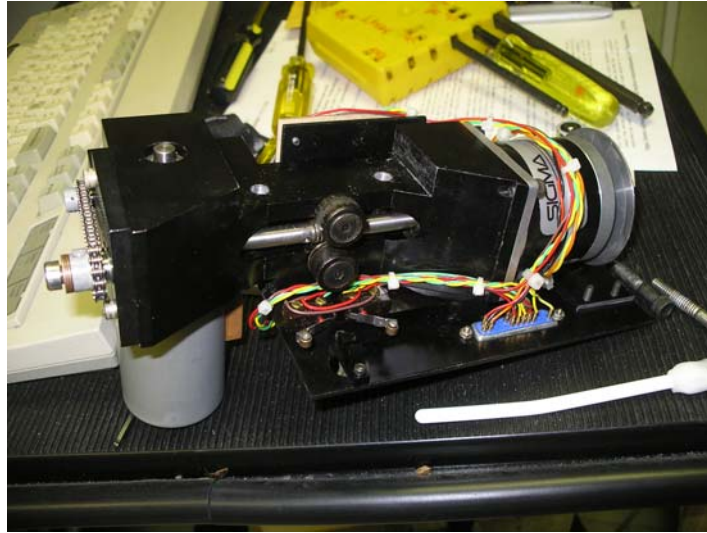
Figure 14: The Blue Channel grating tilt motor assembly removed from the instrument. The worm gear and idler wheels are in the center of the image. The limit switches are near the bottom of the assembly.
