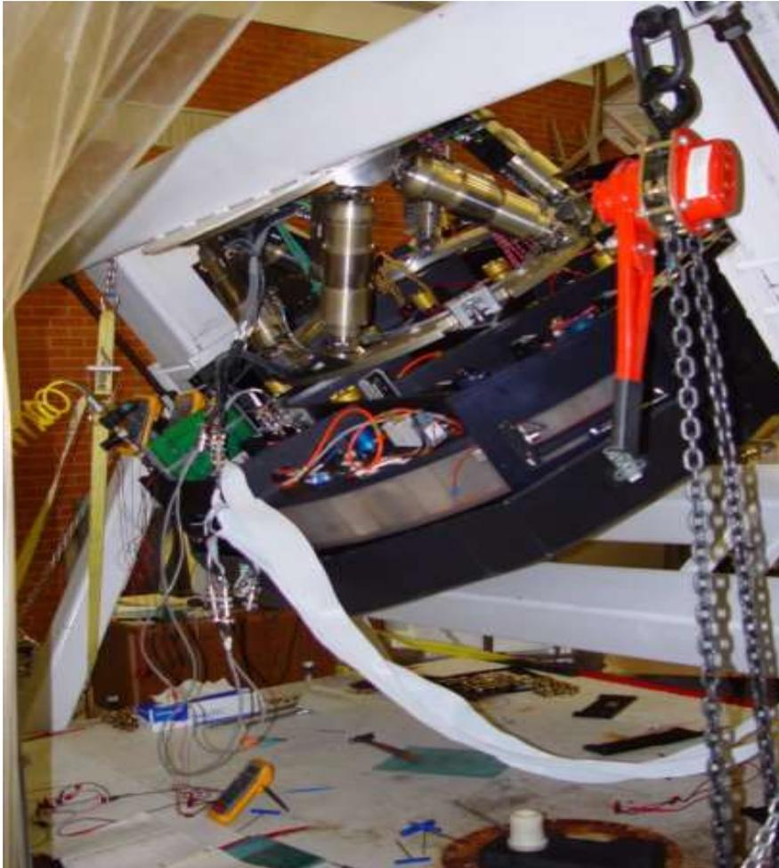
*The image above shows the secondary cell and hexapod assembly on the test platform. This platform, affectionately known as the "Iron Maiden," allowed 180 degree rotation of the assembly as well as precise adjustment of the mirror support system and calibration of the hexapod support electronics. Image by S. Callahan.*
