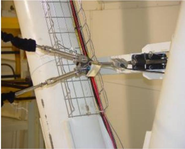
*Figure 3: The east baffle attachment.*
