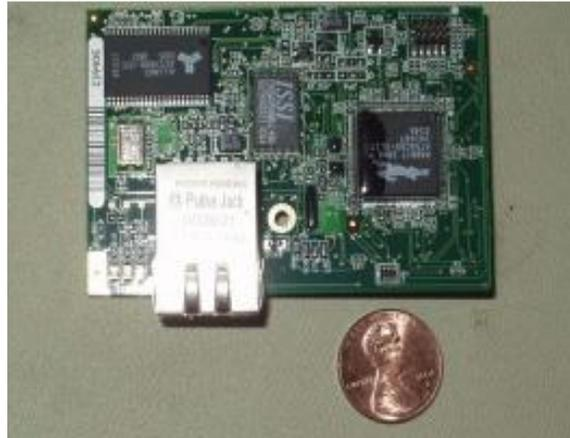
*Figure 5: The Rabbit core module with Ethernet connection.*
