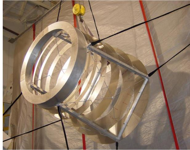
*Figure 4: The mid-baffle fully preloaded on the telescope.*
