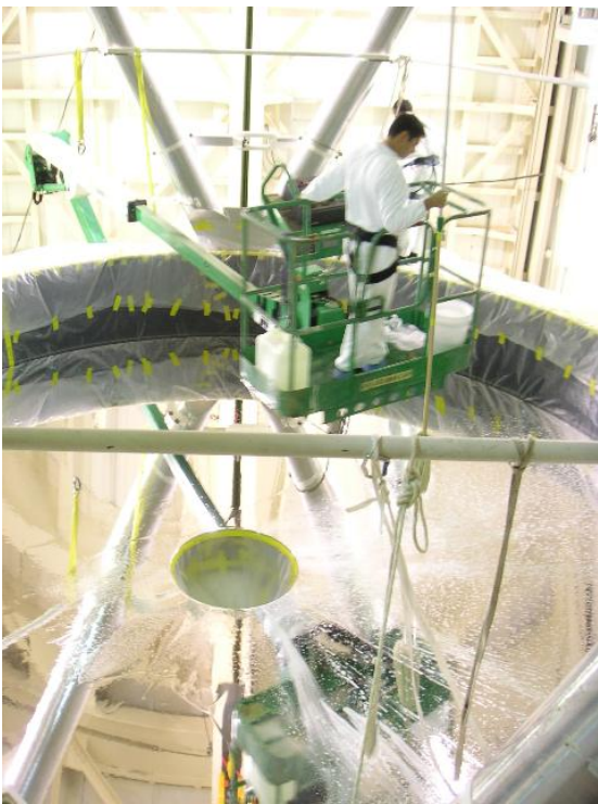
R. Ortiz maneuvers over the primary mirror while “dabbing” the surface with a soapsuds-filled large cotton swab.
