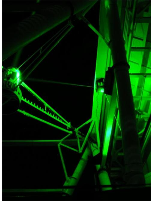
*Two views of the MMT during tests of the Rayleigh laser beacon. Left: the view from the bowl. Right: the laser beam transfer optics — the laser, mounted on the west side of the OSS, fires forward to the pupil optics box on the head frame, then across the telescope beam path to projector optics in the secondary hub, then to the sky. Photos by D. Blanco.*
