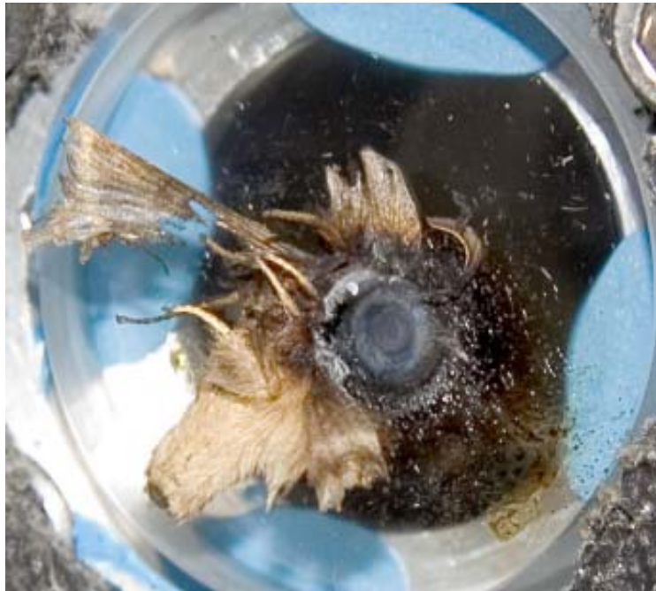
Figure 5: An unfortunate moth flew into the laser beam at the steering prism, bonding to the glass surface.
