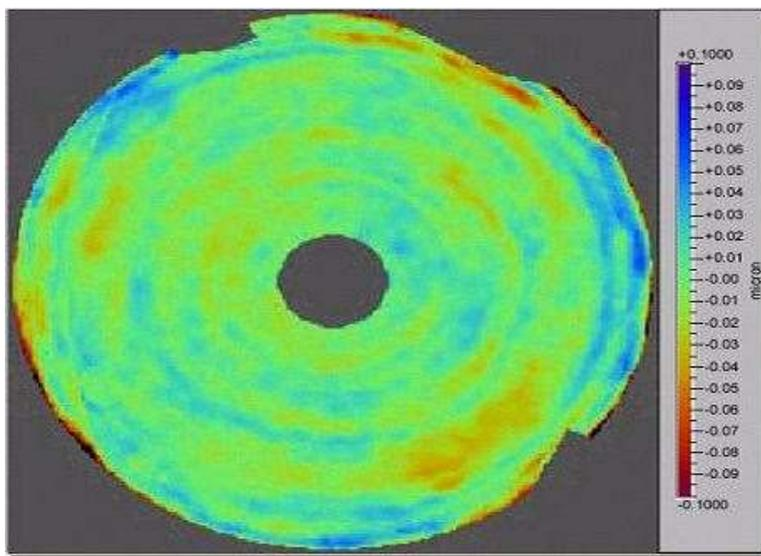
*Map of the surface errors of the completed f/5 secondary – rms error = 17 nm.*
