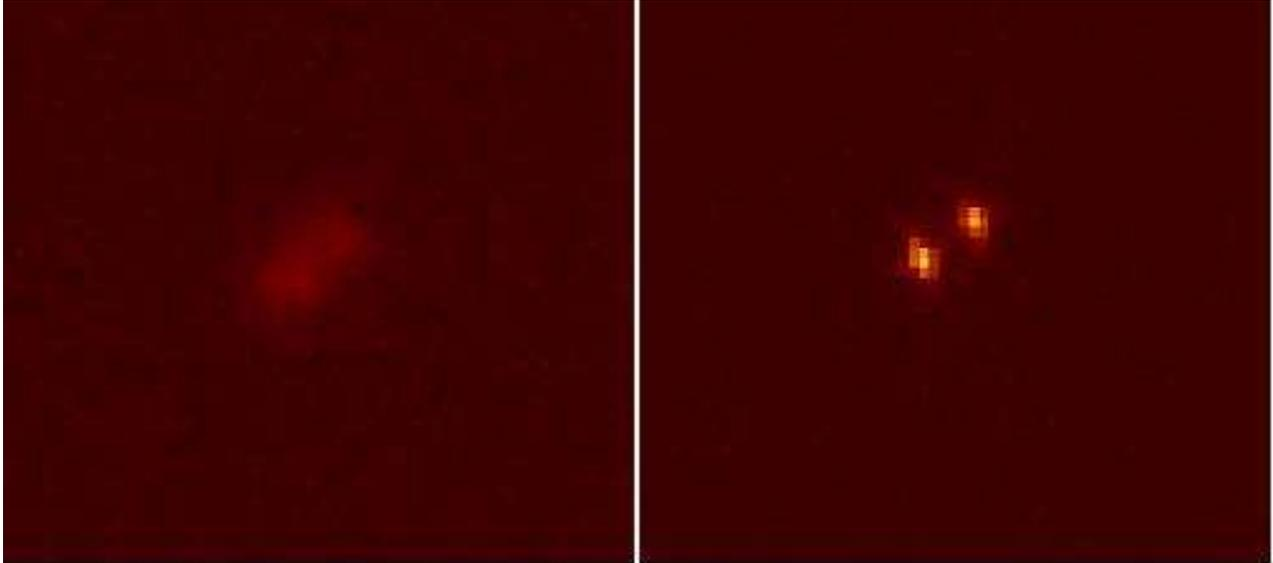
*Figure 1: Here are two 300s duration exposures of the same objects taken in K-band (2.2 micron) with MIRAC. This is the same 0.5 arcsec binary as pictured above, as seen without AO (left) and with AO. Strehl ratio is approximately 10%.*
