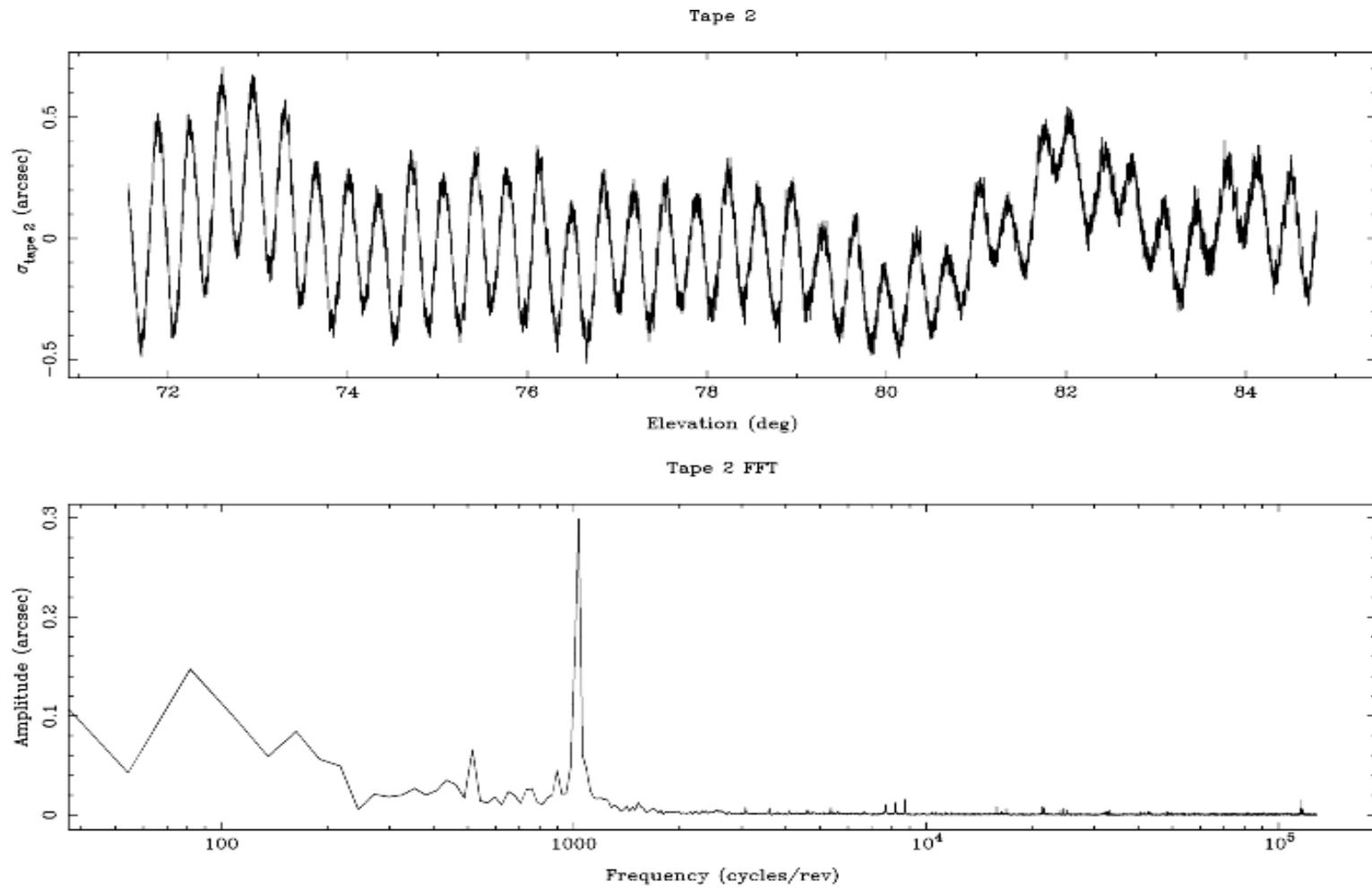
Figure 3: Plot of elevation tape readout with outer loop closed. Note the prominent peak at 1024 cycles/rev with a smaller, but still significant, peak at 512 cycles/rev.
