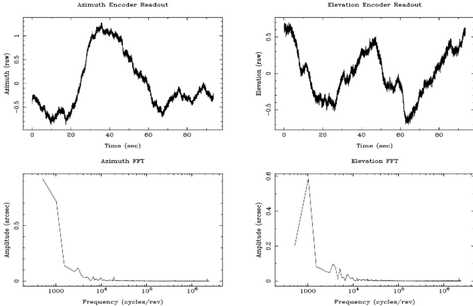
Figure 2: Plot of detrended indexer readout over a single 0 to 65535 count cycle. The indexer cycles 512 times per 360 degrees of revolution, so the 1024 cycles/rev oscillation cycles twice per indexer cycle. This is clearly seen on the elevation readout. The outer loop was open for this test, which results in the significant mechanical noise that is likely washing out the 1024 cycles/rev signal in the azimuth output.
