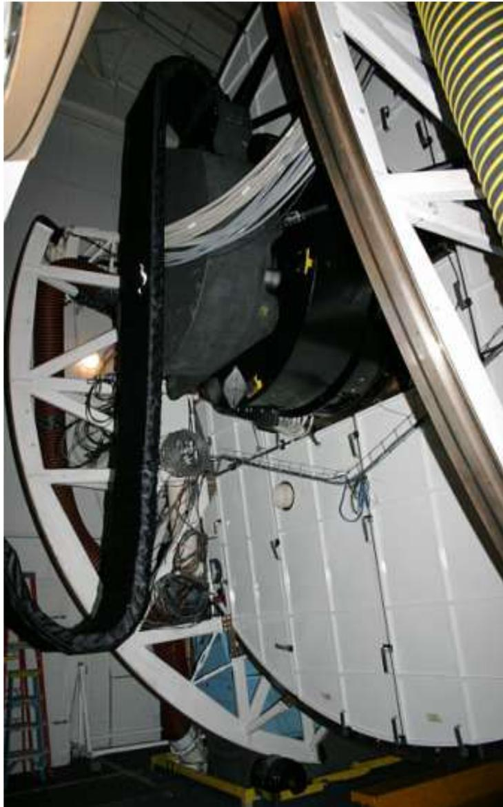
*The fiber positioner mounted on the nearly horizon-pointing telescope during the October Hectospec commissioning run. The fiber bundle, containing 300 fibers, runs inside the black S-shaped energy chain. (Image by D. Fabricant.)*
