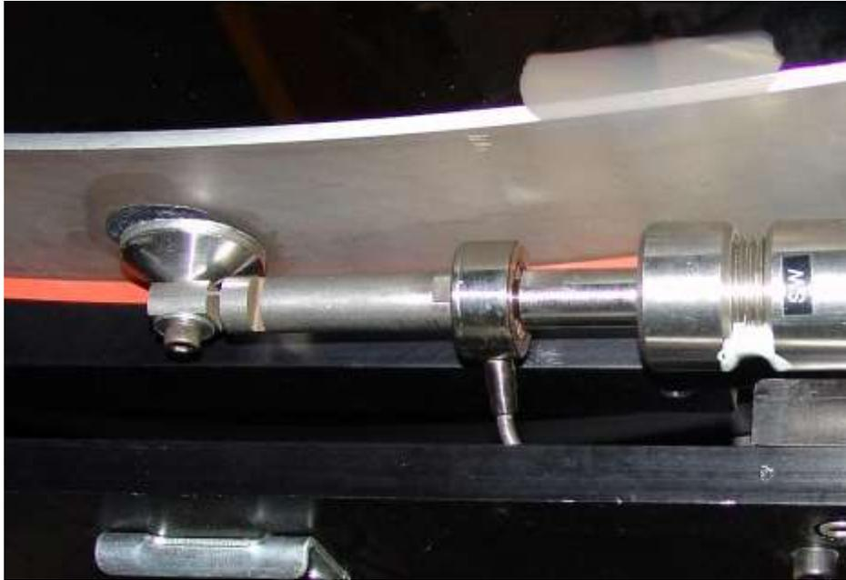
*Figure 2: One of two ruptured glue bonds (two-part RTV, Q3-6093).*
