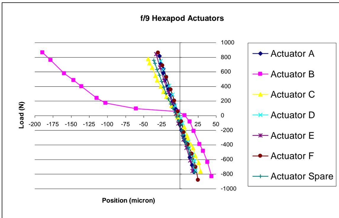
Figure 1: Stiffness testing results of  $f/9$  hexapod actuators.
