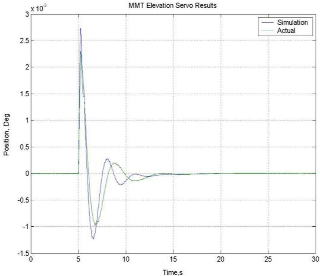
Figure 4: Closed-loop step disturbance response.
