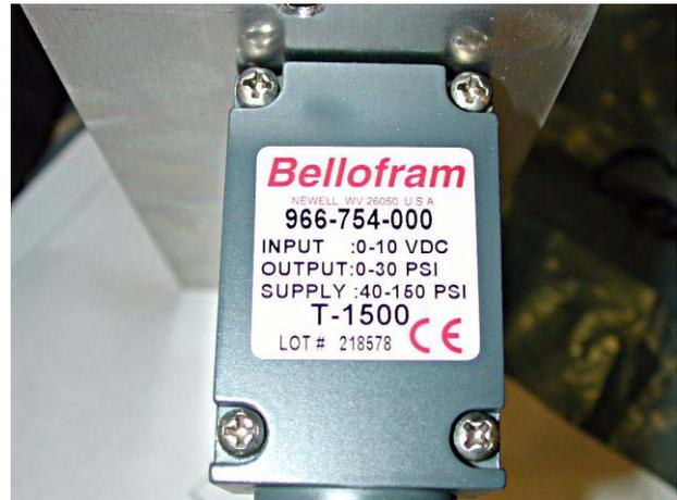
Figure 8: Photo identification of one of the 4 air regulators currently used in f/9 mirror support system.
