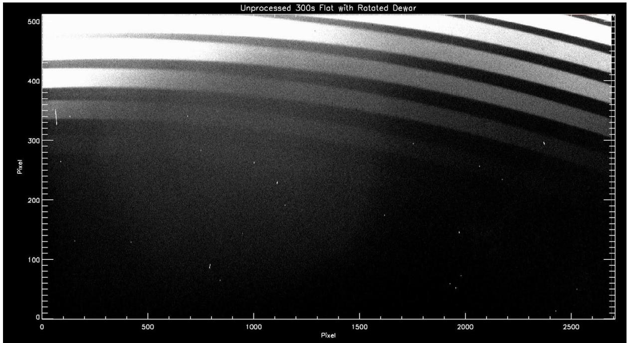
It's clear from this image that the rotation only worsens the problem. At this point, no simple correction will extend the coverage of the Blue Channel echellette to the red while not simultaneously adversely affecting non-cross dispersed observations.
