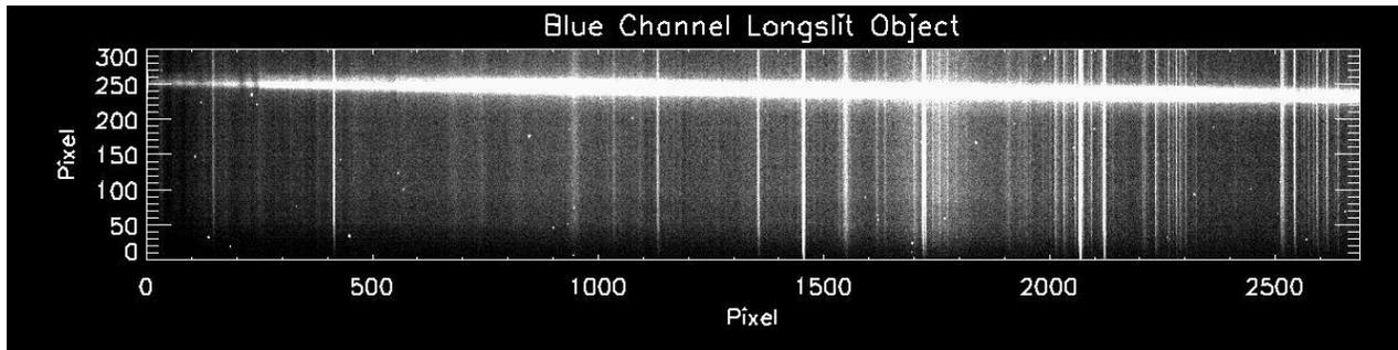
At the bottom of this image, one can see that the brightness (both in the lines and sky continuum) fade in brightness as they approach pixel 0. This occurs as the current CCD placement in the dewar is such that it is not perfectly centered on the middle of the spectrograph slit - the bottom of the image is imaging the end of the slit.
