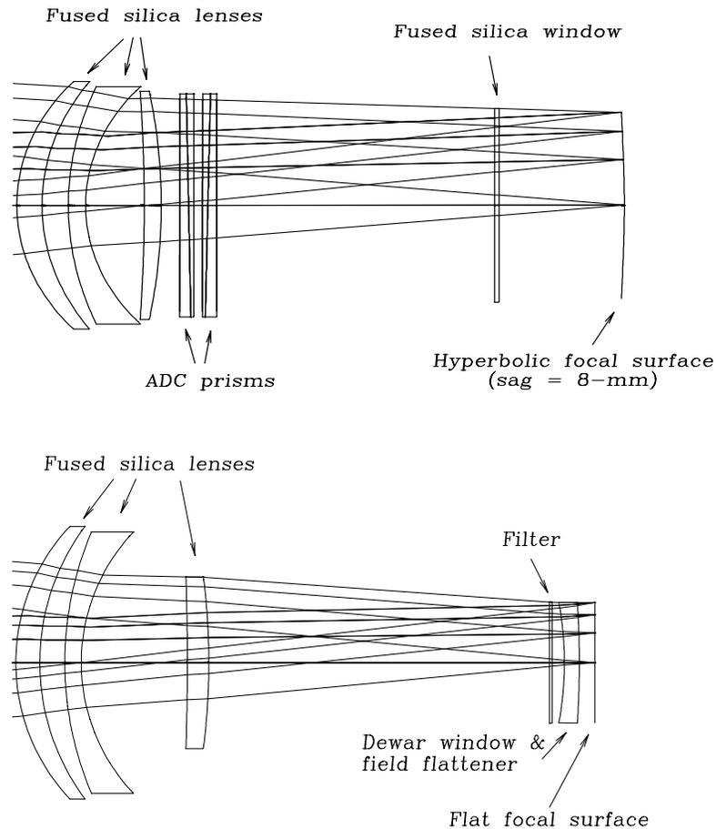
**FIGURE 3. The two  $f/5.4$  wide field imaging modes of the 6.5-m MMT. The top view is for wide-field spectroscopy and the bottom for imaging.**
