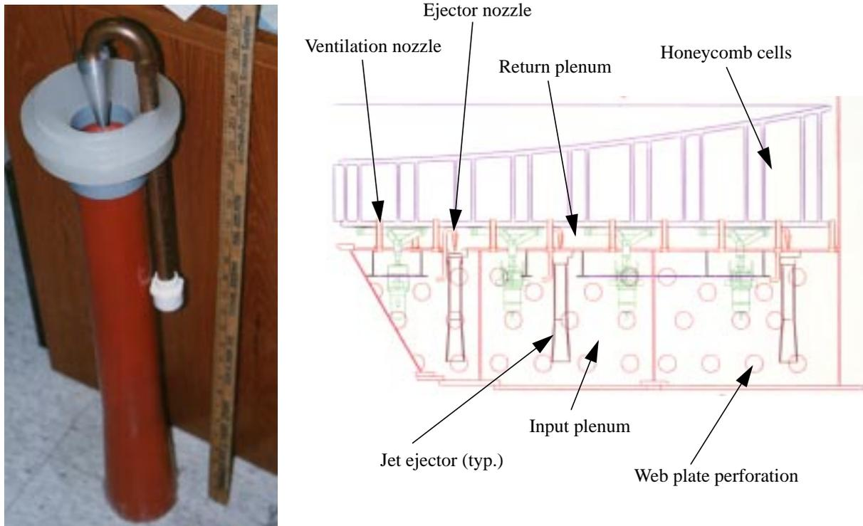
**FIGURE 9. A prototype jet ejector for thermal control of the primary mirror (left). At right is a schematic of the thermal system contained in the primary mirror cell.**
