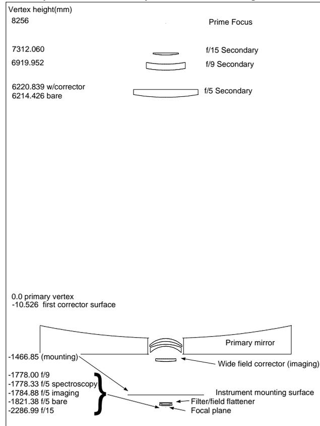
**FIGURE 2. Cassegrain optical configurations for the 6.5-m MMT .**
