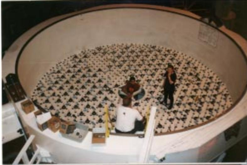
**FIGURE 5.** The zenith-pointing 6.5-m mirror cell in the Steward mirror lab. Seen are most of the 200 static supports (they define the set of axial and lateral resting forces for the mirror when the active support system is turned off) and the 1100+ ventilation air nozzles which squirt air into the interiors of the mirror honeycombs and around the mirror periphery. The vacuum seal flange is visible near the ID of the top of the trunnion ring.
