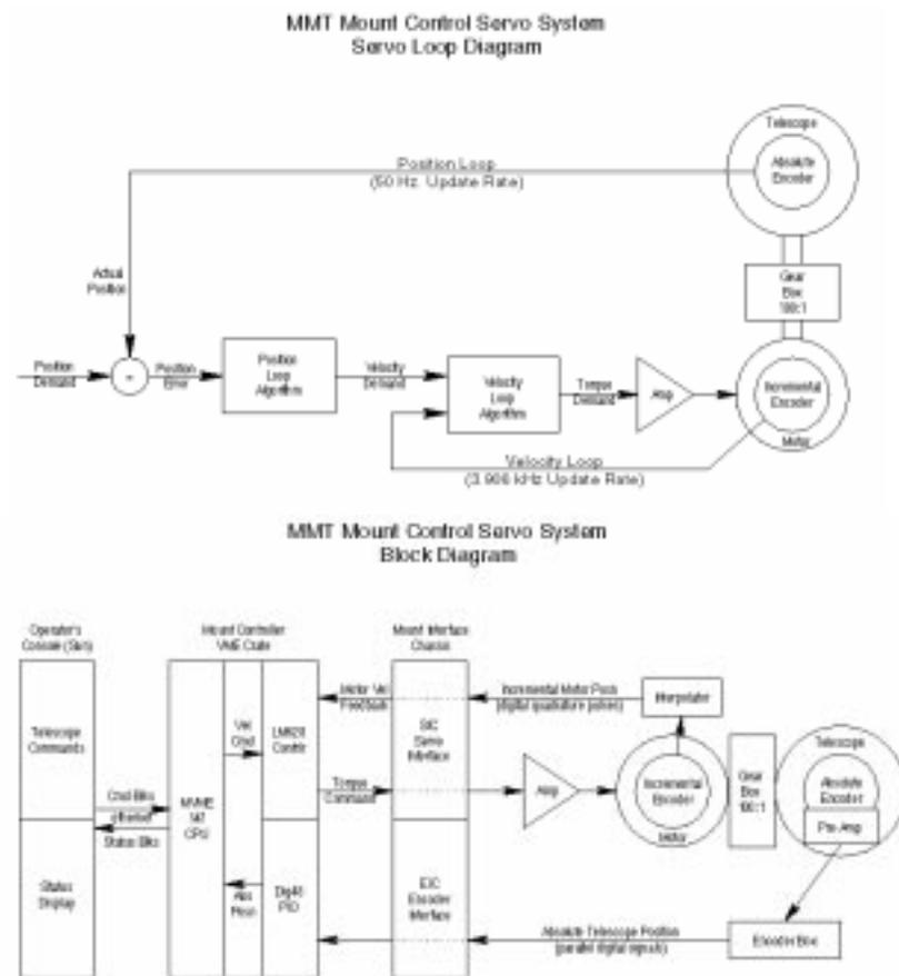
**FIGURE 10. Schematics of the MMT servo control system. See text for details.**
