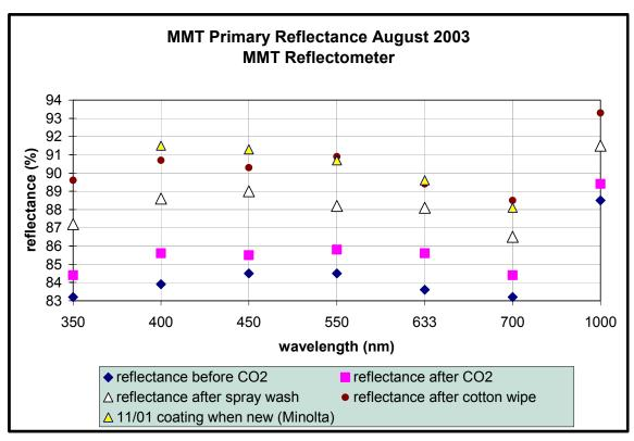
Figure 1. Reflectance at various stages of cleaning.
