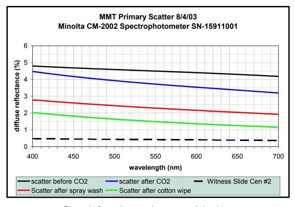
Figure 1. Scattering at various stages of cleaning.
