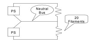
Figure 1 Typical Filament Circuit (1 of 5)
