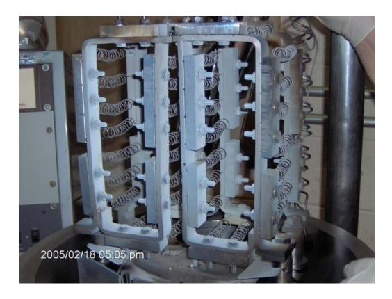
Figure 5. Test Fixture After Firing
