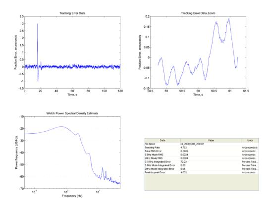
This file reports a peak-to-peak error of just over 4 arcseconds, due to the offset step response at ~18s. The RMS error seen in this file is reported as 0.14", yet if only the data from 20s to the end is processed, the RMS error becomes 0.067" – a much more reasonable result, given the obviously smaller amplitude in the majority of the time history.
