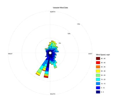
The wind speed intensity and wind azimuth values from the Python filter operation is shown above. The *Vaisala 3* sensor has since been repaired, and we await more data from it as a check on the *Vaisala 4* output.
