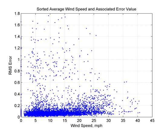
Clearly, a few poor tracking entries exist for all wind speeds in the data, and most of the good tracking is clustered at wind speeds below ~15mph.
