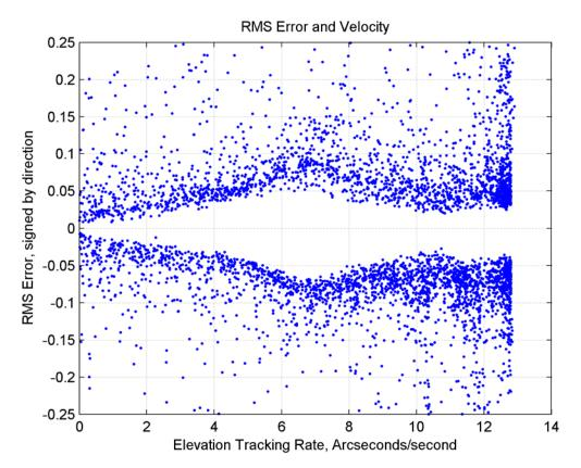
Tracking smoothness appears unaffected by the tracking direction, but cannot go below about  $\pm 2$  encoder counts. In addition, the tracking error shows a non-linear dependence on the tracking rate. Work on encoder feedback improvements (i.e. improved alignment, period counting) would help make this lower limit on tracking error smaller.
