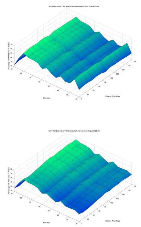
Next, we have these graphs of the relative wind angle and intensity, with the same averaged RMS error in the z-axis, for both guarded and unguarded data:
