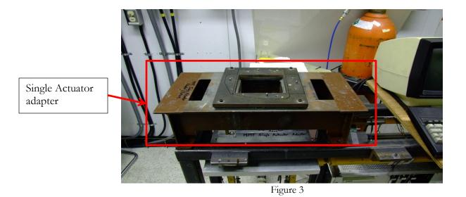
Figure 3 shows the single actuator assembly. This part is one solid piece that attaches to the teststand frame via 4 bolts. It is clearly marked on the surface which direction the adapter faces and where it should lay on the frame. Once this piece is attached, single actuators may be affixed for testing and calibration.
