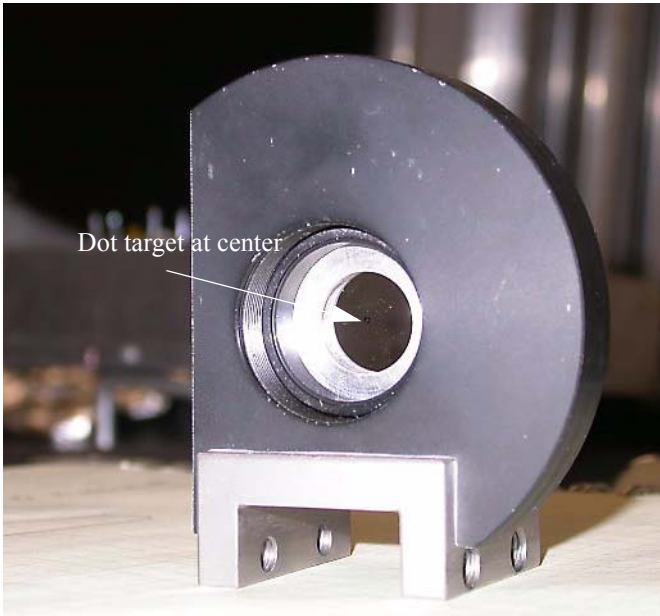
Figure 16: Remove the optics from the 1:1 reimager optical path, so that the above rail target can be slid along the entire length of the X-26 rail.
