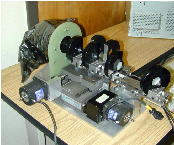
Figure 6: The as-built f/9 Shack-Hartmann wavefront analyzer prior to installation in the top box.
