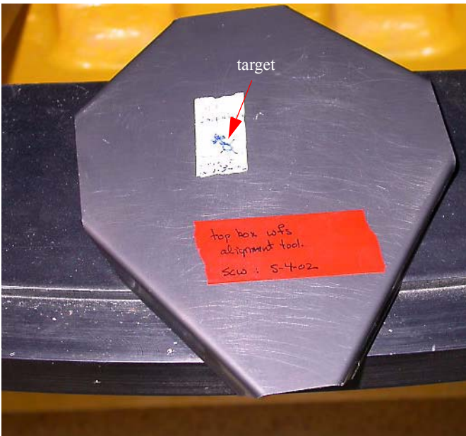
Figure 13: Move in comparison assembly. Snap on mirror cover shown in figure. Laser should intersect target. Remove cover. This is a sanity check that the mirror is positioned properly and that the laser is on-axis.
