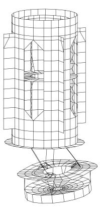
If we consider a hexapod interface made of aluminum instead of steel, its weight decreases from 89.8 daN to 30.9 daN. In such conditions the *Optical System* always weighs 206.2 daN; meanwhile the *Complete System* weighs 407.7 daN.
