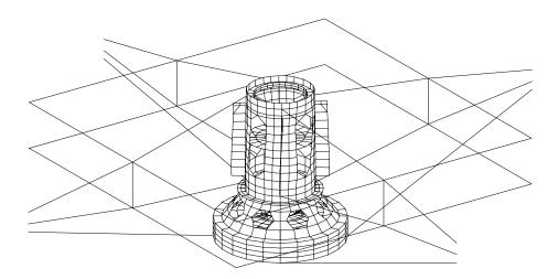
Second mode shape: Hub piston, 24.3 Hz
