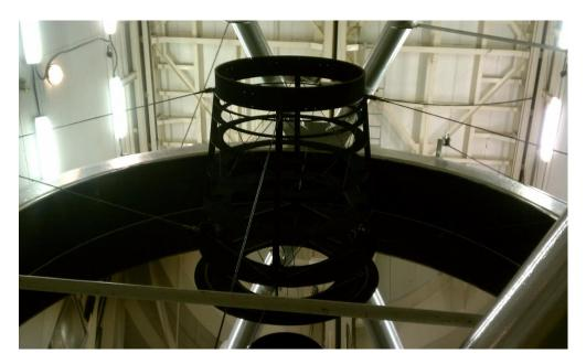
Figure 1. Mid-baffle extended at zenith.
