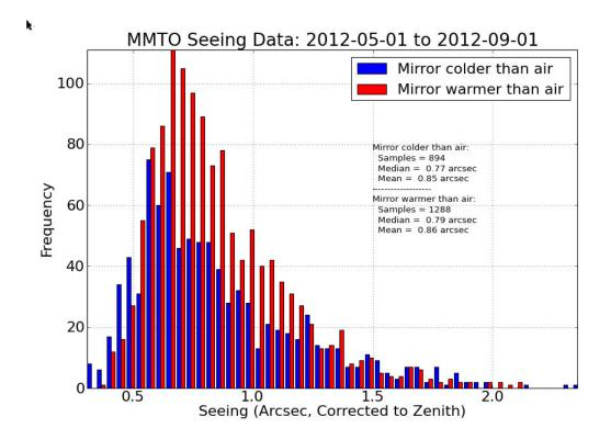
Figure 17. Seeing values under different M1 glass-air temperature conditions. The data plotted in blue represent seeing values when the mirror is colder than the adjacent chamber air temperature. The data in red were obtained when the mirror glass was warmer than the adjacent air temperature. The latter case is unfavorable since local mirror seeing is introduced at the glass-air interface under these conditions.
