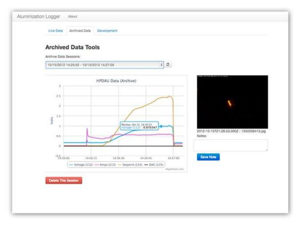
Figure 11. Screenshot of the archive viewer for data recorded from aluminization tests.
