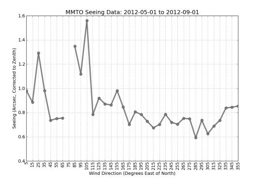
Figure 18. Median seeing variation with respect to wind direction for May through August 2012. No seeing measurements were made at a wind direction of 75° east of north during this period. In general, seeing is degraded when the wind is from the east and improved when the wind is from the south to west.
