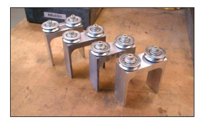
Figure 5. Machined pulley brackets for mid-baffle synchronization system.
