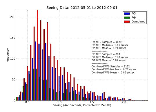
Figure 16. Histogram (with 0.1 arcsec bins) of derived seeing values for the f/5 and f/9 WFSs from May through August 2012. Seeing values are corrected to zenith. Median f/5 seeing is 0.81 arcsec while the median f/9 seeing is 0.70 arcsec. A combined (f/5+f/9) median seeing value of 0.78 arcsec is found for the 2,182 WFS measurements made during this period.
