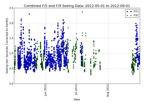
Figure 15. Derived seeing for the f/5 and f/9 WFSs from May through August 2012. Seeing values are corrected to zenith. The f/5 seeing values are shown in blue while f/9 values are in green. A median seeing of 0.78 arcsec is found for the 2,182 WFS measurements made during this period.
