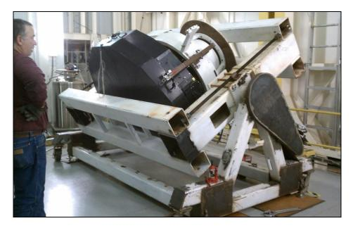
Figure 4. f/5 secondary on test stand at 45 degrees.
