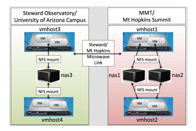
Figure 7. Host computers, virtual machines (VMs), and network-attached storage (NAS) devices now in use at the MMT Observatory on Mt Hopkins and at the MMT offices at Steward Observatory on the University of Arizona campus.
