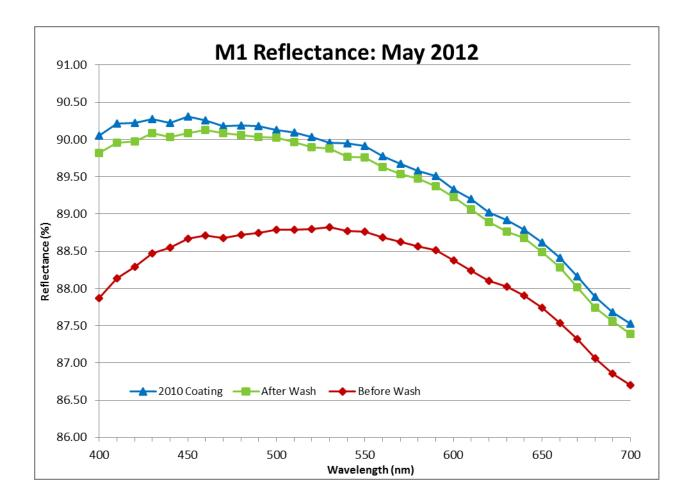
Figure 1. M1 Reflectance: May 2012, before and after wash, compared with 2010 coating.
