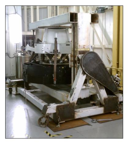
Figure 3. f/5 secondary on test stand at nadir pointing.
