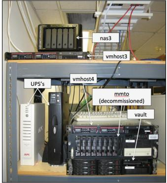
Figure 9. VM host computers, NAS boxes, and uninterrupted power supplies (UPS's) on the 3rd floor of Steward Observatory, on the campus of the University of Arizona. See text for additional details.
