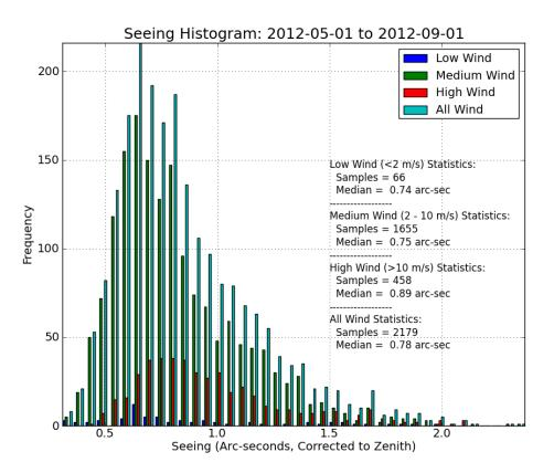
Figure 19. Histograms (with 0.1 arcsec bins) of seeing within different wind speed ranges for May through August 2012. For "low" and "medium" wind speeds, defined as <2 m/s and 2-10 m/s, respectively, the median seeing is approximately 0.75 arcsec. For high wind speeds (above 10 m/s), seeing is substantially worse with a median value of 0.89 arc-sec.
