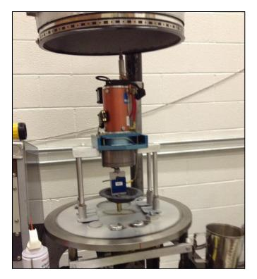
Figure 4. An M1 single axis actuator in the small Sunnyside chamber.
