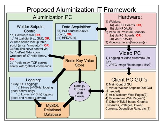
Figure 5. Proposed information technology (IT) framework for the MMTO primary mirror (M1) realuminization effort.
