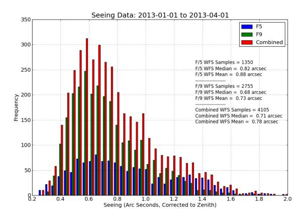
Figure 13. Histogram (with 0.1 arcsec bins) of derived seeing values from the f/5 and f/9 WFS for January through March, 2013. Seeing values are corrected to zenith. Median f/5 seeing is 0.82 arcsec while the median f/9 seeing is 0.68 arcsec. A combined (f/5+f/9) median seeing value of 0.71 arc-sec is found for the 4,105 WFS measurements made during this period.
