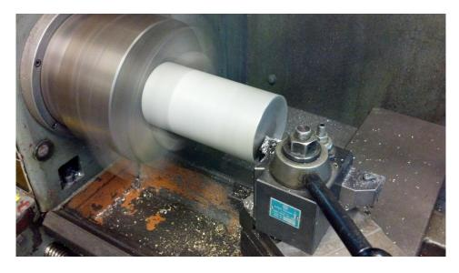
Figure 1. Rough cutting aluminum stock to be used for the test tool.
