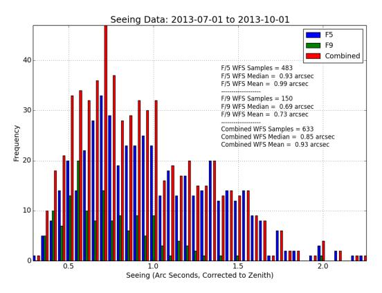
Figure 6. Histogram (with 0.1 arcsec bins) of derived seeing values for the f/5 and f/9 WFSs from July through September 2013. Seeing values are corrected to zenith. Median f/5 seeing is 0.93 arcsec while the median f/9 seeing is 0.69 arcsec. A combined (f/5+f/9) median seeing value of 0.85 arcsec is found for the 633 WFS measurements made during this period.
