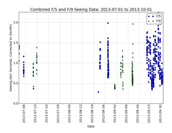
Figure 5. Derived seeing for the f/5 and f/9 WFSs from July through September 2013. Seeing values are corrected to zenith. f/5 seeing values are shown as blue circles while f/9 values are shown as green triangles. An overall median seeing of 0.85 arcsec is found for the 633 combined (f/5 and f/9) WFS measurements made during this period.
