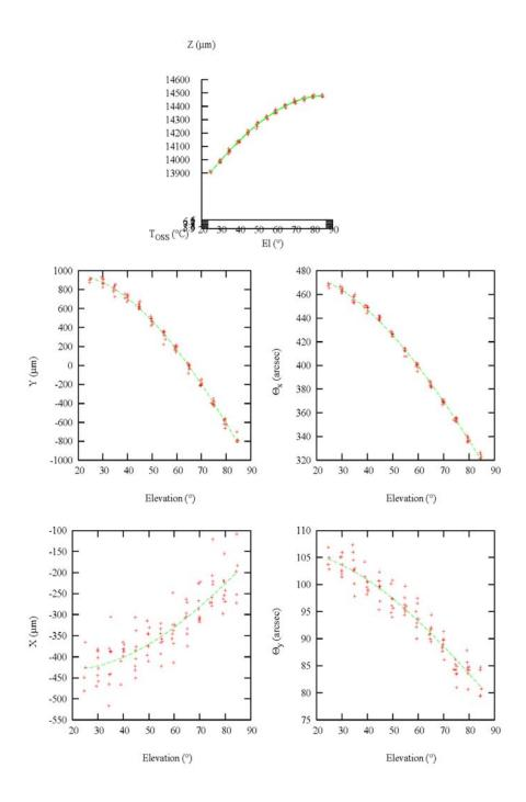
Figure 1: Results of engineering data taken with the f/5 WFS on the night of April 25-26, 2006, showing the elevation dependence of the five axes of M2 motion. The plot of Z vs. Elevation is tilted slightly to de-project the temperature dependence.
