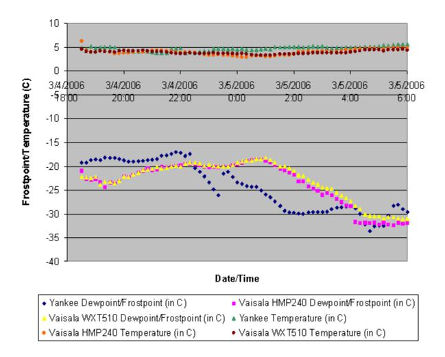
Figure 5: Comparison of dewpoint temperature measurements from three units for the night of March 4-5, 2006.
