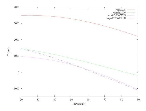
Figure 3: Y vs. Elevation relations determined at different times between November 2005 and late April 2006. Note the very large offset of about 2.5 mm between November 2005 and all of the results from 2006.
