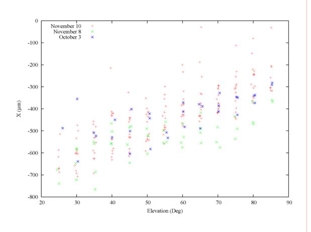
Figure 3: X-translation vs. elevation from engineering data taken in October and November 2006
