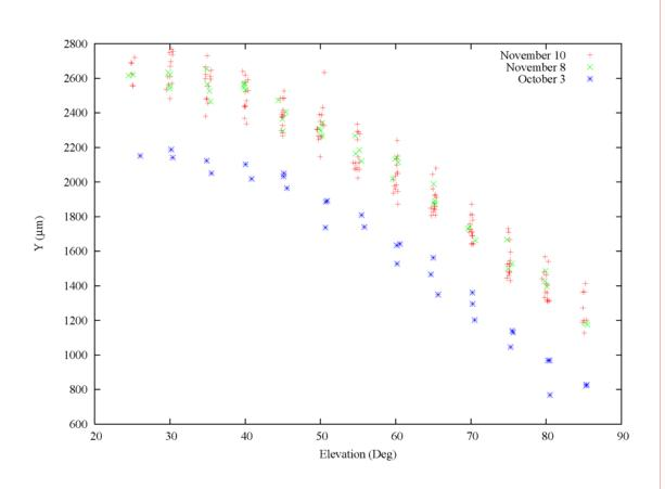
Figure 2: Y-translation vs. elevation from engineering data taken in October and November 2006
