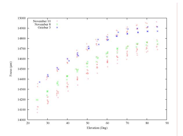
Figure 1: Focus vs. elevation from engineering data taken in October and November 2006
