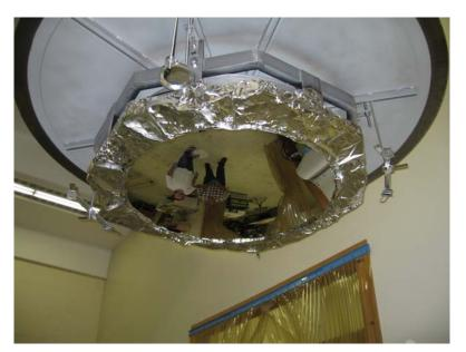
Top left: Chemically stripped of its old aluminum coat, the lightweight f/9secondary is shielded from adjacent mirror support hardware, likely sources of contamination during the vacuum pumping viscous phase.
