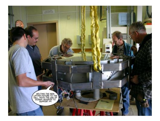
Figure 1: Bill Stangret (right) operates a hydra-set lift, lowering his new multi-purpose logistics frame onto the f/9 secondary mirror and its telescope cell. Ricardo Ortiz, Mike Alegria, J. T. Williams, and Dennis Smith give the new tool a favorable review. Photo by John Glaspey (MMTO).
