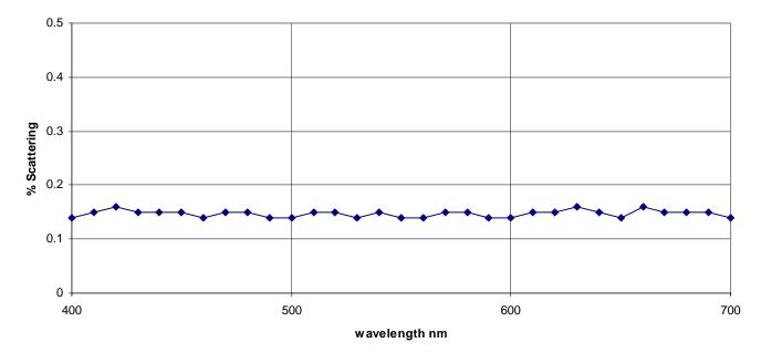
Figure 2b: Scattering plot for the center of the f/9 secondary following the October re-aluminization. Measured with Minolta Spectrophotometer #CM-2002.
