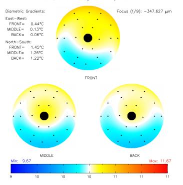
Figure 3: Results of analyzing primary mirror thermal structure during the night of October 29. The data were taken at 1:22 UT (top left), 4:25 UT (top right), and 8:29 UT (bottom). Each plot shows the results of polynomial surface fits to Eseries temperature data for the front, mid, and back plates. The diametric gradients are determined directly from the fits and the focus error is determined from the fits in combination with FEA models.
