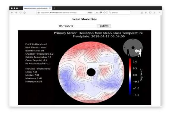
Figure 2. A "birds-eye" view of thermal gradients across the M1 mirror, similar to Figure 1, but showing increased thermal gradients across the mirror. These data were taken from a night in which the telescope chamber remained closed due to weather conditions. Strong thermal gradients in the primary mirror can impact image quality and require larger wavefront-sensor corrections.
