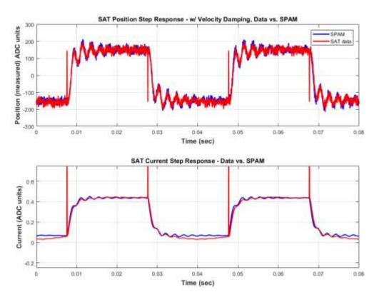
Figure 3. Step response comparison of hardware test fixture results with simulation prediction for position and current.
