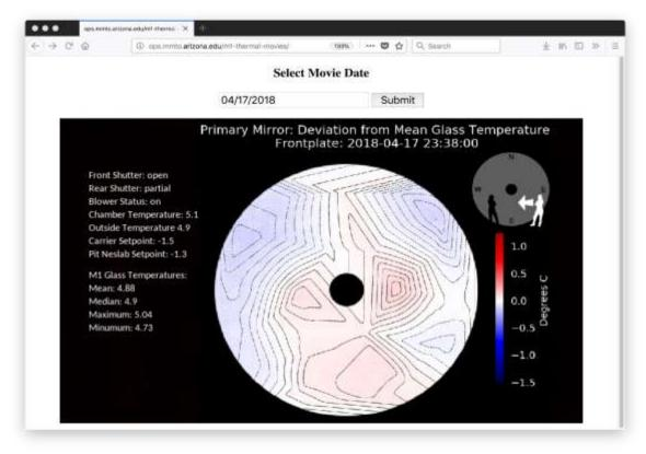
Figure 1. A "birds-eye" view of thermal gradients across the M1 mirror. Contour lines show the deviation from the mean glass temperature. The maximum gradient across the mirror is around 0.3°C in this screen capture, indicating that the mirror is nearly isothermal.
