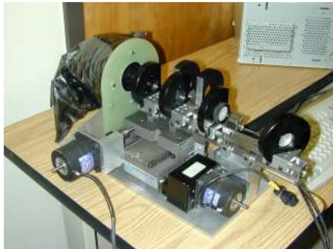
Figure 4: Photo of the f/9 top box wavefront sensor prior to inserting the optics.
