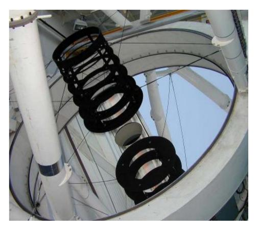
The lower baffle deployed. Photo by C. Wainwright.
