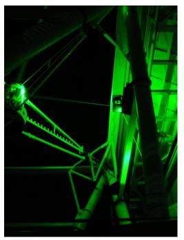
Two views of the MMT during tests of the Rayleigh laser beacon. Left: the view from the bowl. Right: the laser beam transfer optics — the laser, mounted on the west side of the OSS, fires forward to the pupil optics box on the head frame, then across the telescope beam path to projector optics in the secondary hub, then to the sky. Photos by D. Blanco.
