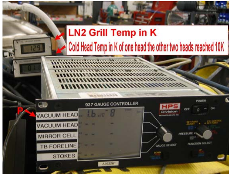
Figure 3: Ultimate pressure testing of #1 cryopump at Austin Scientific.
