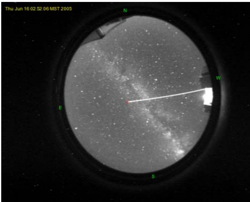
An all-sky camera image of a laser beam during the June 14-18 Laser Guide Star observing run at the MMT.
