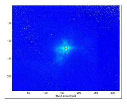
H-band image taken with the f/15 secondary. Adaptive loop not closed.
