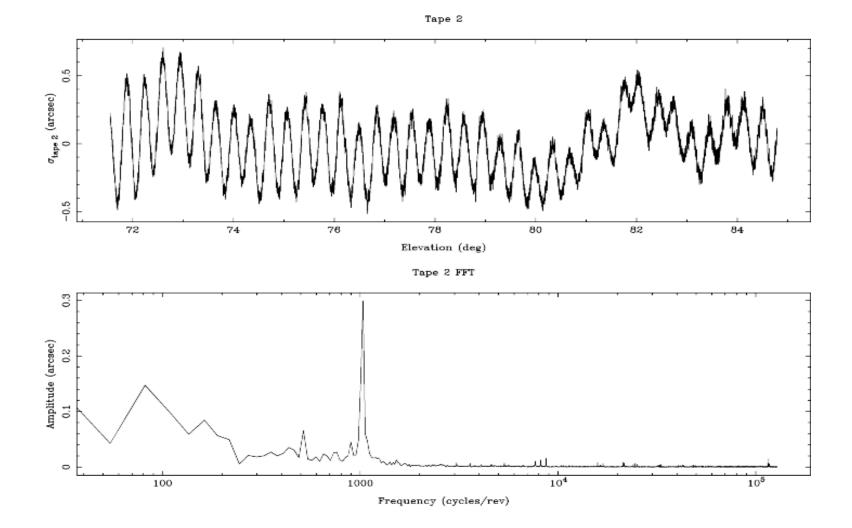
Figure 3: Plot of elevation tape readout with outer loop closed. Note the prominent peak at 1024 cycles/rev with a smaller, but still significant, peak at 512 cycles/rev.
