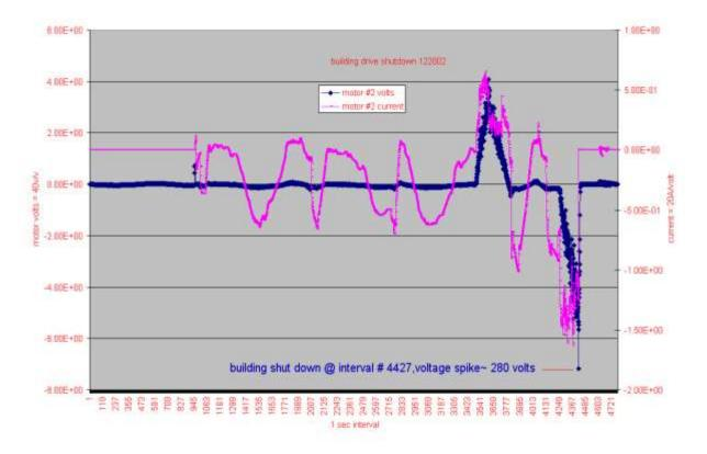
Figure 4: Building drive motor voltage monitored during a shutdown.
